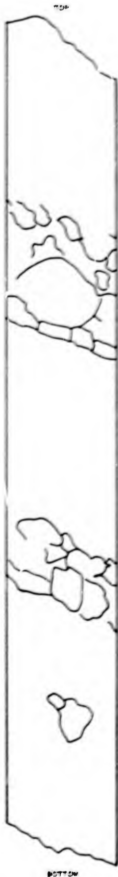
Grain boundaries in gneissic, anhydrite-bearing salt, dipping 25 to 30 degrees. Depth: 2698.5-2699.5 ft, core NMC-13, hole 4, Tatum Dome
