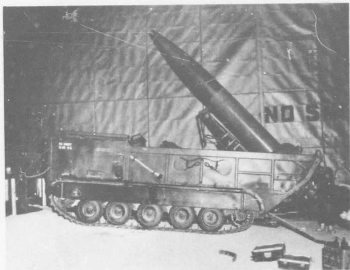
Fig. 1 Side view of Self-propelled Launcher, showing emergency tools and recesses used for climbing into the cab.
