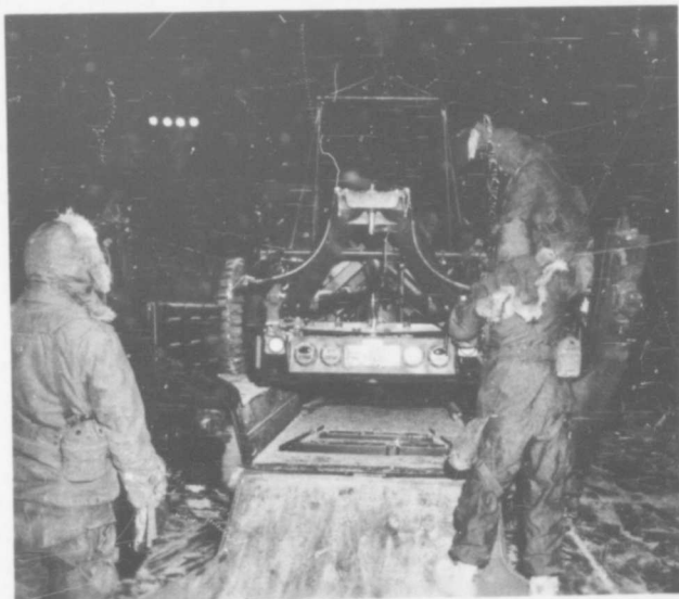
Fig. 4 Rear view of Self-propelled Launcher, showing slippery ramp.
