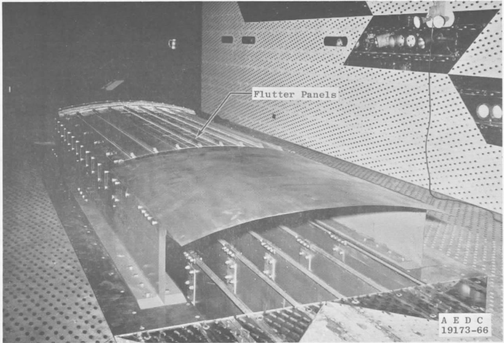
Fig. 3 Photograph of Flutter Model Installed in Tunnel 16T
