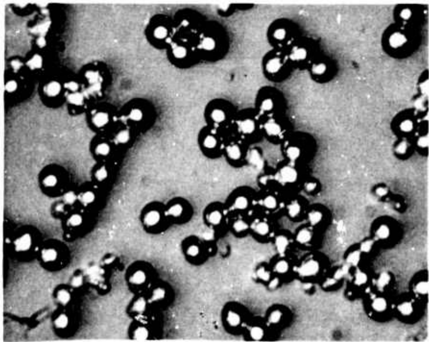
Figure 9. Photomicrograph of Union Carbide Powder Lot UC-3 Showing the +20% Powder Fraction. X1000
