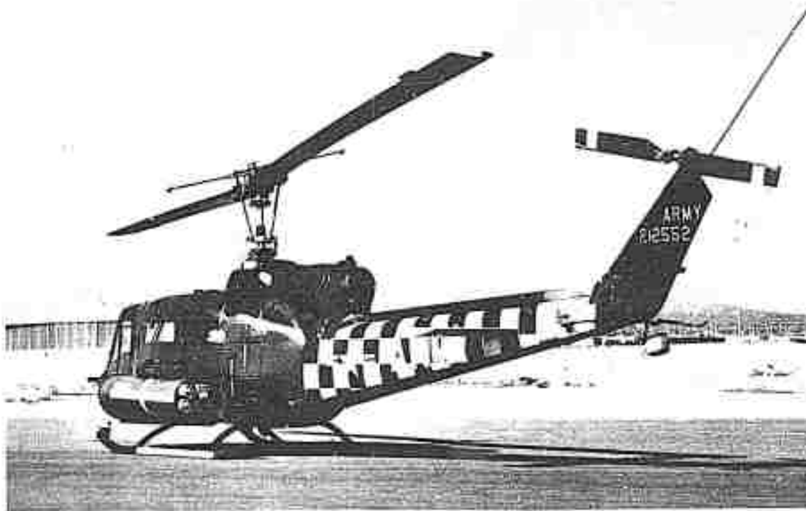
PHOTO 2 - Left rear view of UH-1B having left XM-3 Dispenser loaded with four XM-2 Antipersonnel Mines and tail skid camera
