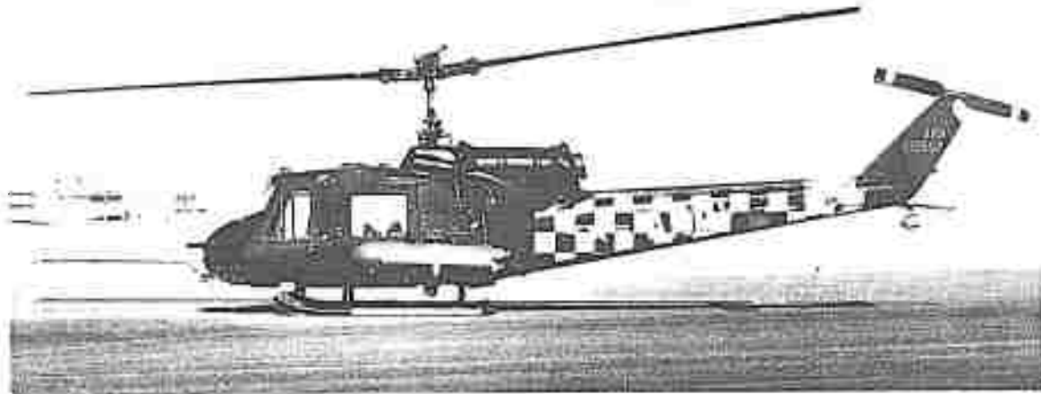
PHOTO 1 - Left side view of UH-1B with XM-3 Dispenser
