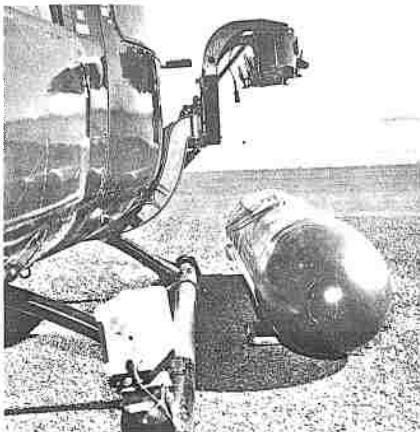
Photo 5 UH-1B with Kellet Mounts on standard universal external pylons, unmounted XM-3 Dispenser and skid camera.
