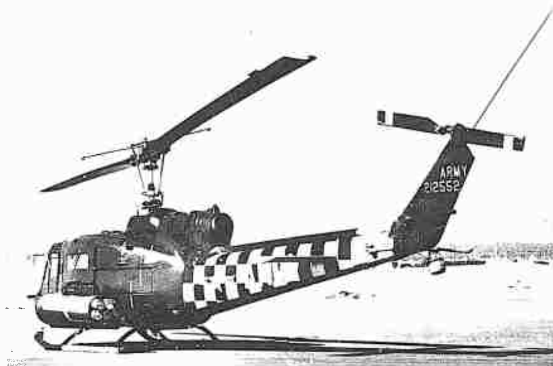
Photo 2 - Left rear view of UH-1B showing left XM-3 Dispenser loaded with four XM-2 Antipersonnel Mines and tail skid camera.
