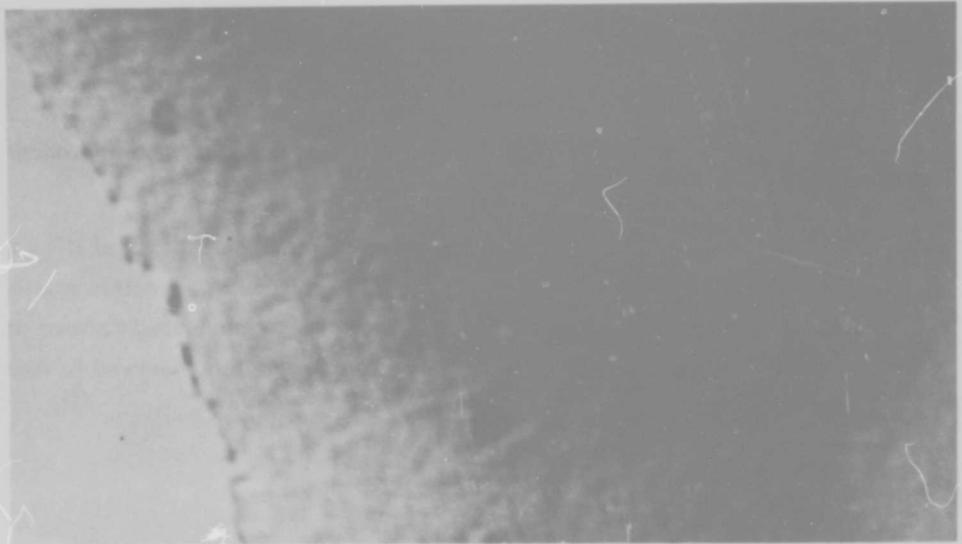
Fig. 67 Another Example of the Textured Appearance of Thinned Boron Filament. 183,000 \times . P1493-4a
