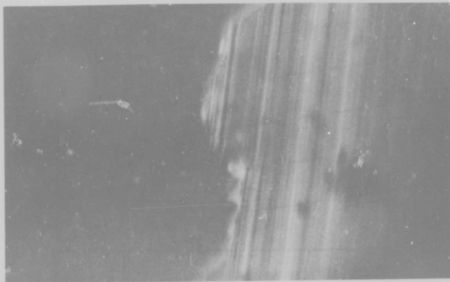
Fig. 87b Dark Field Image of Same Area, Showing Illuminated Striations. 31,500 \times , P923
