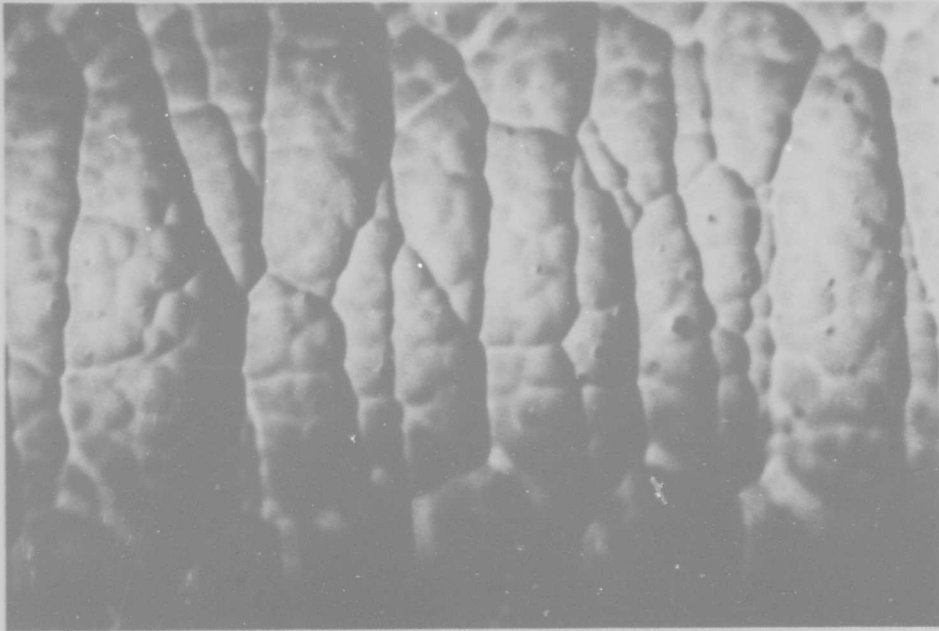
Fig. 5(a) Surface of Texaco-1 Filament. M9013, 3000×
