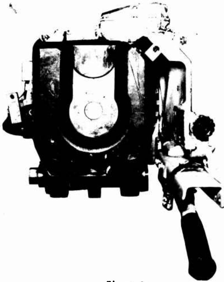
Figure 8 Breech Block For M32 Cannon Modified To Clear The Mount For The M81E12
