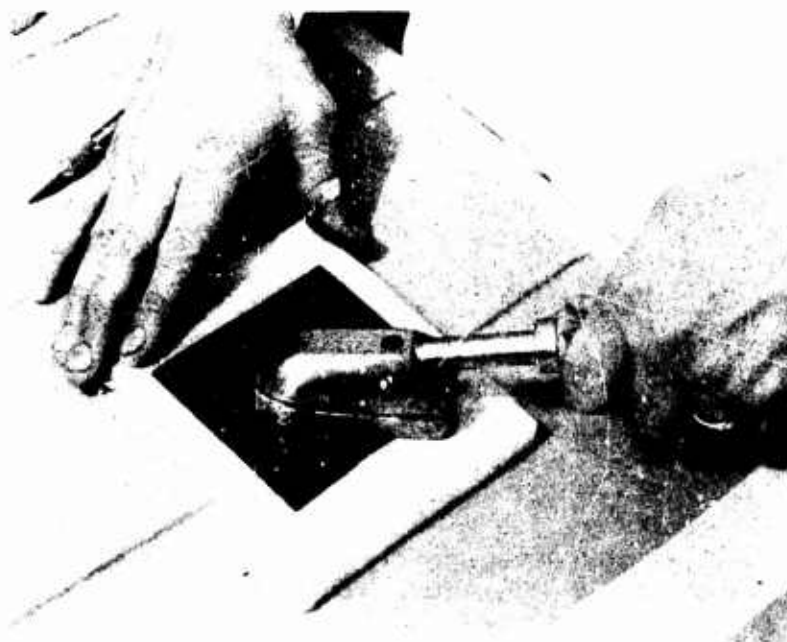
Figure 3. Tacking double ply with hot iron. Mylar film prevents resin from sticking to iron. (HAC Photo No. R109188)
