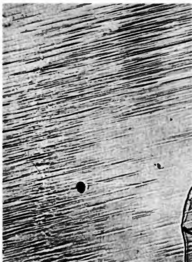
Figure 13. Slip Lines in Mo 2 C (32.5 At% C). Alloy Cooled at ~100°C per Second from 1700°C.
