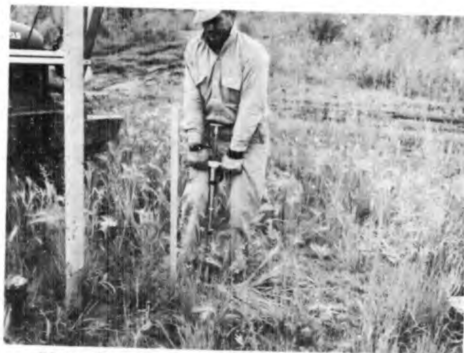
Figure 60. Drive sampling with Hvorslev sampler.
