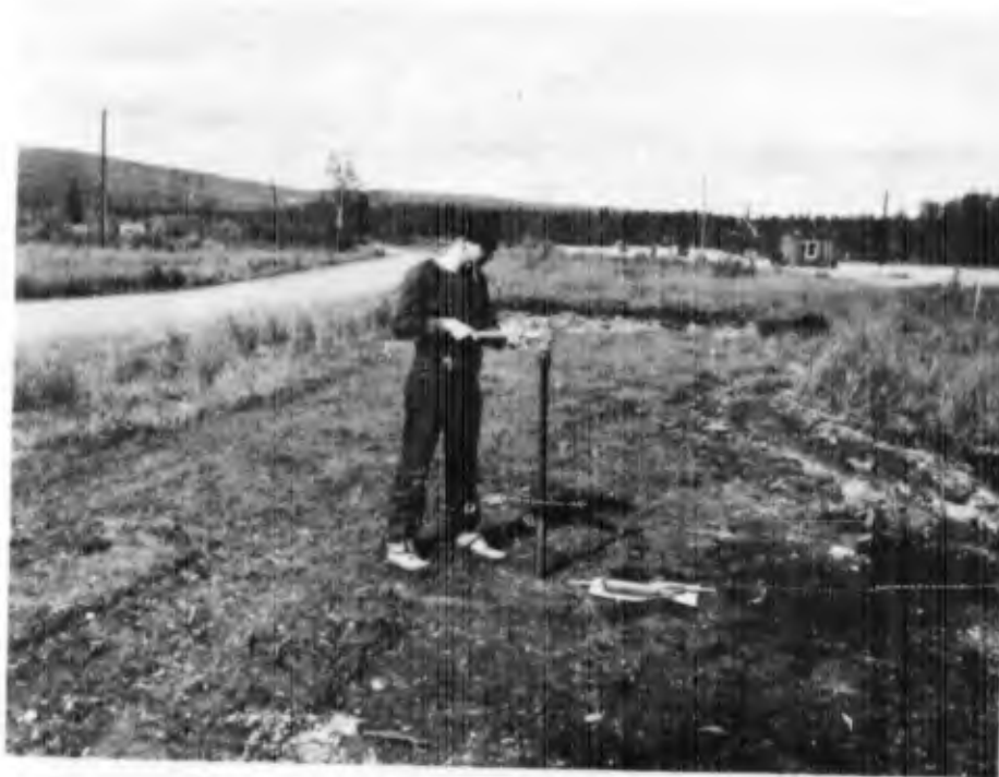
Figure 55. Driving Shelby tube with sledge hammer.
