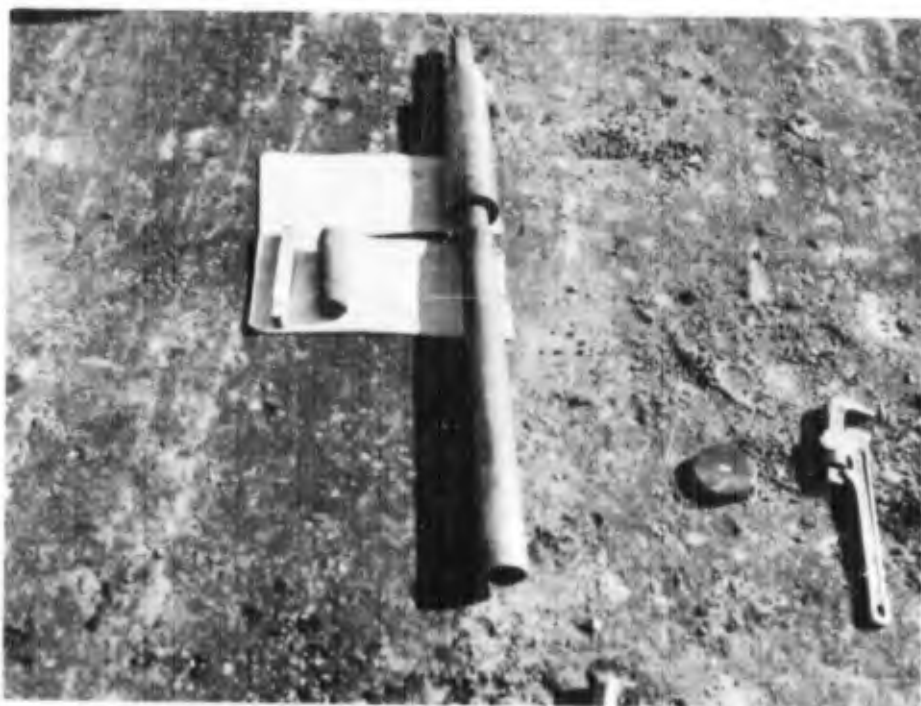
Figure 53. Drive arrangement for shallow soil sampling.
