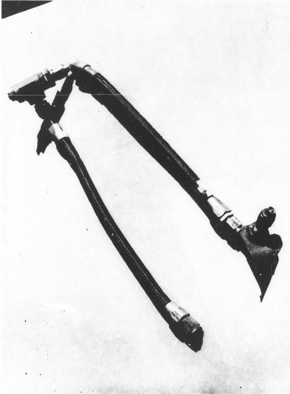
Figure 27. Fitting Failure Caused by Crash Impact.
