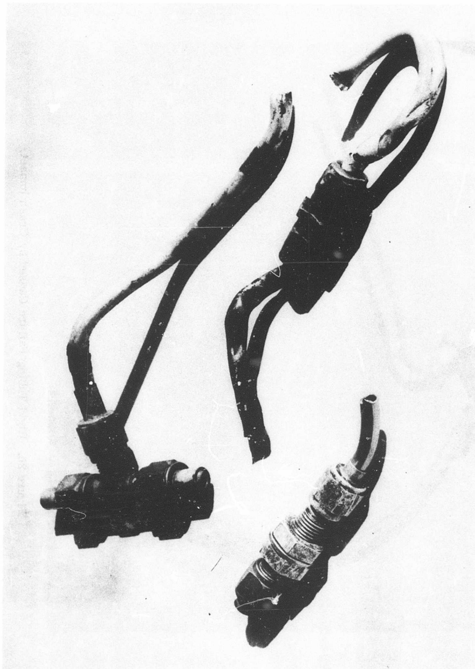
Figure 25. Rigid Tubing Failures Caused by Crash Impact.
