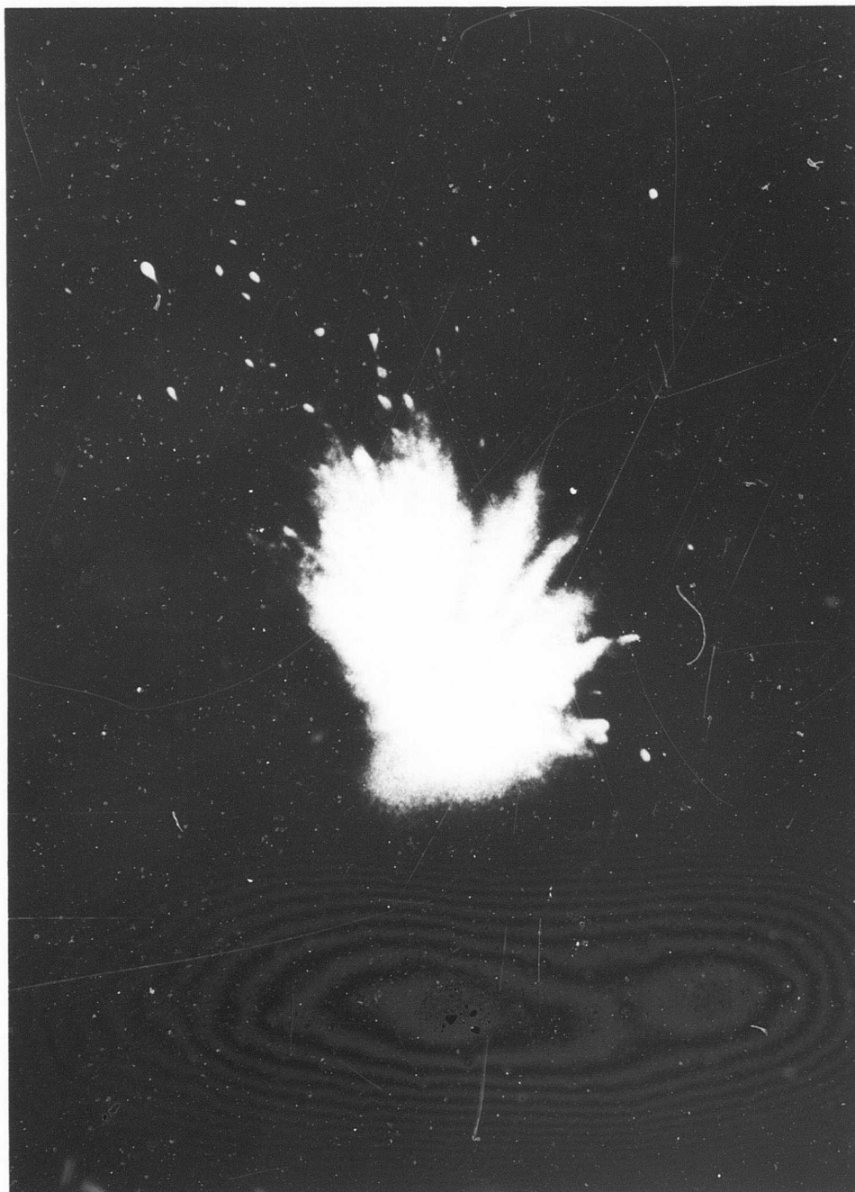
Figure 31. Ballistic Flash Impact From Projectile Penetration of an 0.125-Inch Thick Aluminum Sheet.
