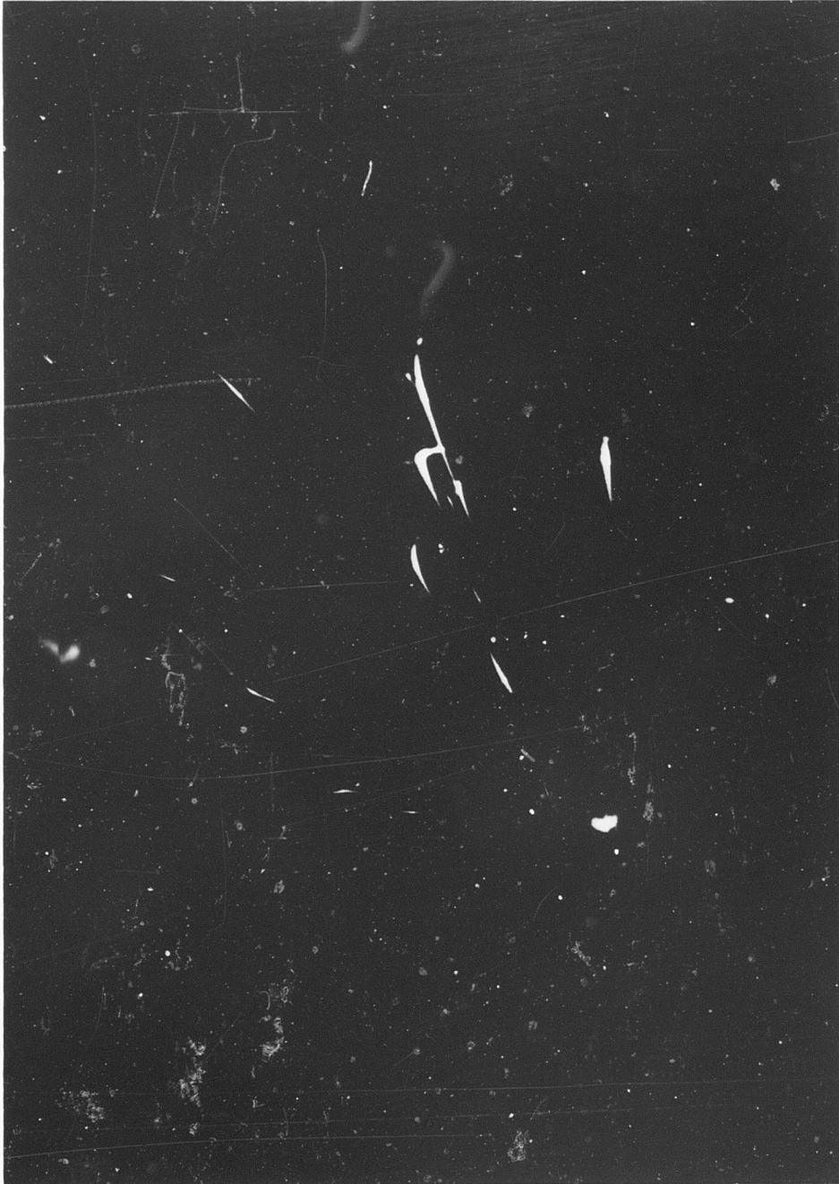
Figure 39. Infrared Photograph, Ballistic Impact Flash of Steel.
