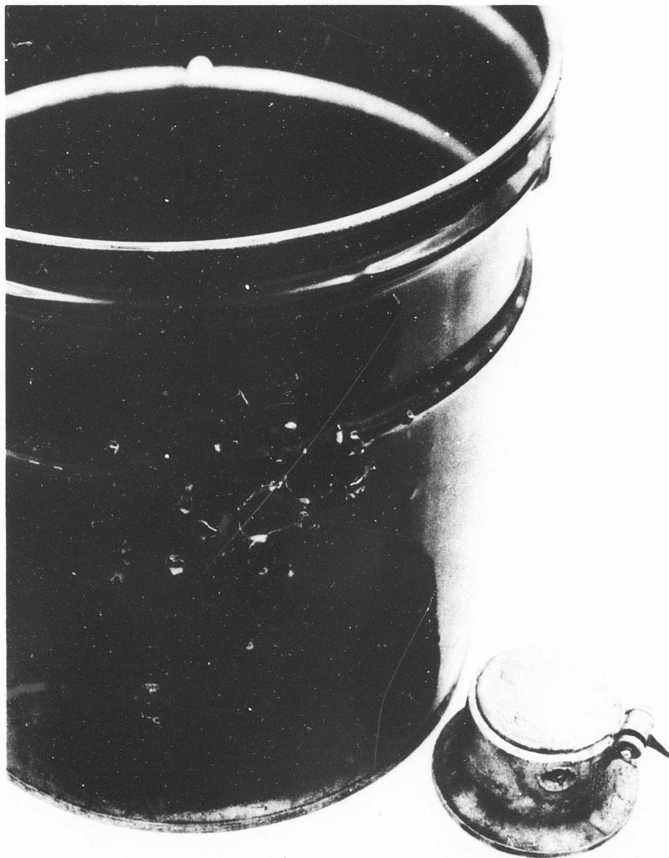
Figure 44. Cast Aluminum Component and Container After a Small Arms Ballistic Hit.
