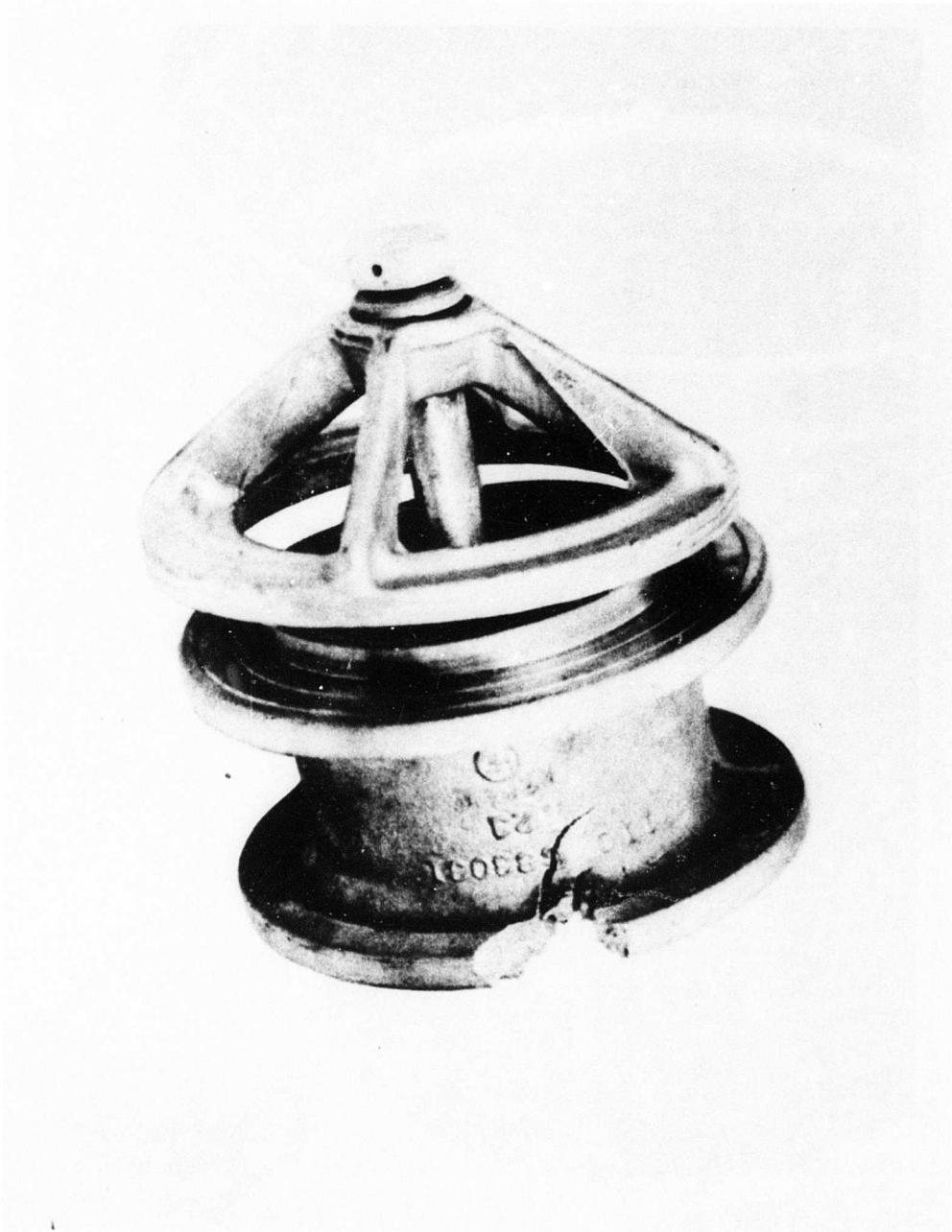
Figure 43. Cast Aluminum Fuel Cell Interconnect After Being Struck by a Small Arms Projectile.
