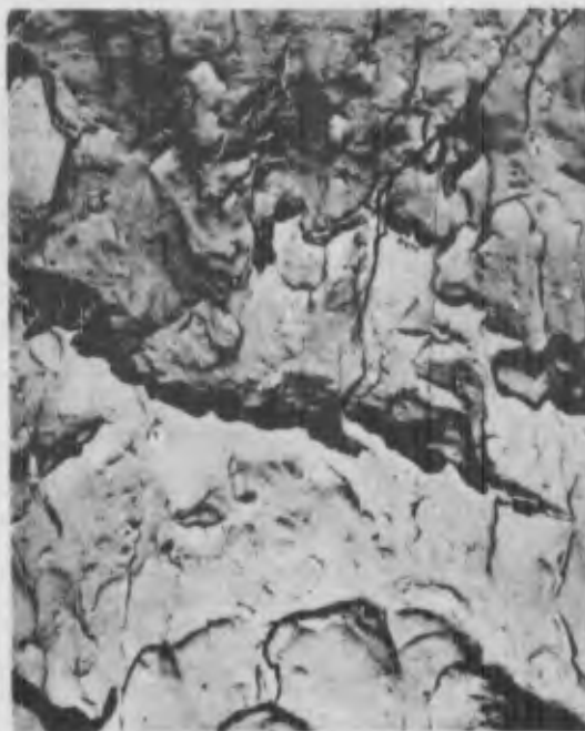
b) Replica A, Fatigue to Slow Growth Region Mag: 3860X
