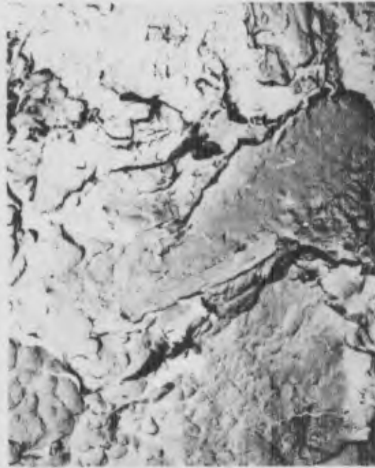
d) Replica B, Slow to Rapid Growth Region Mag: 3860X
