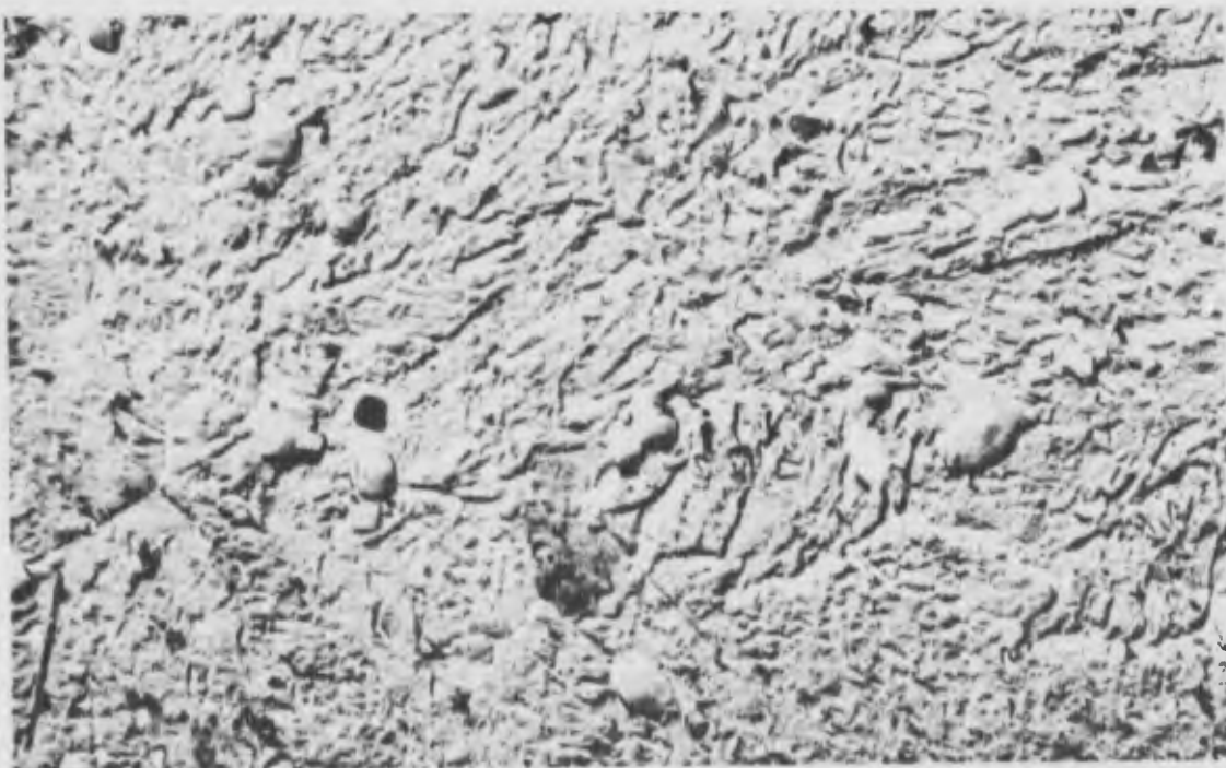
Figure 45. Micrographs of 9Ni-4Co-0.45C bainitically quenched at 550° F (see Table V)
