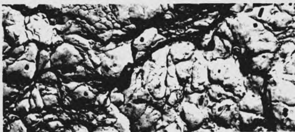
c) Specimen A87, K_{IC} = 88.2 \text{ ksi } \sqrt{\text{in.}} , Heat 3960633.
