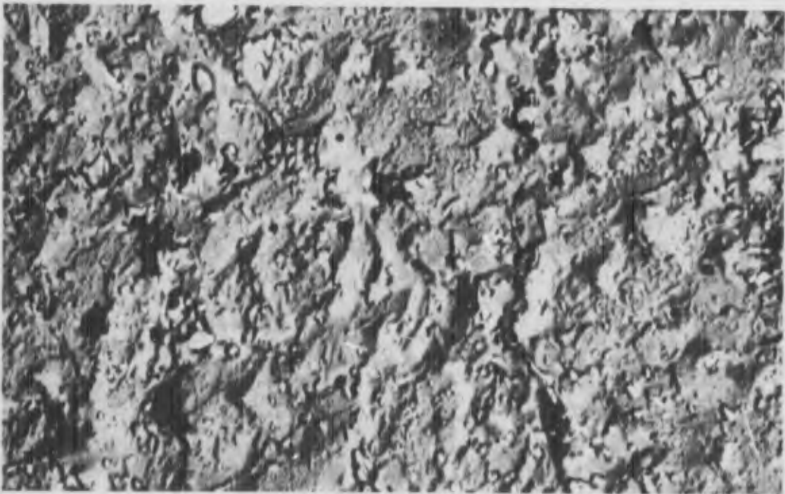
Figure 30. Micrographs of H-11 Modified triple-tempered at 1,175° F (see Table V)
