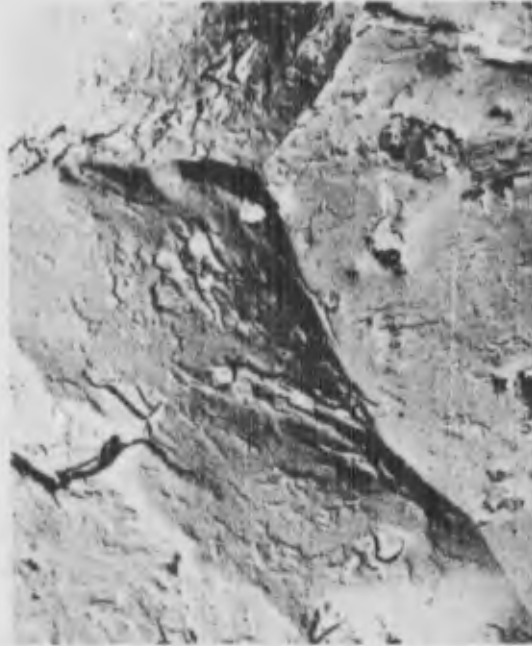
d) Replica A, Intergranular Slow Growth Region Mag: 3860X
