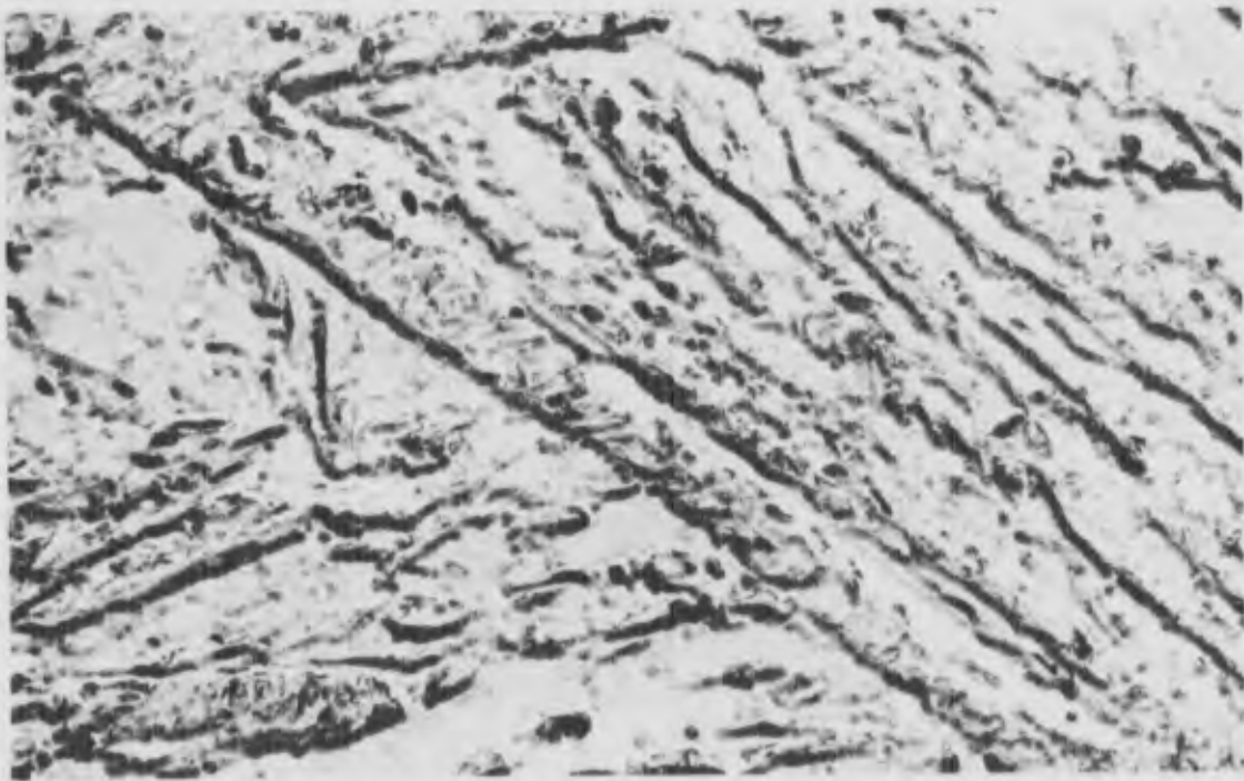
Figure 34. Micrographs of 300M double-tempered at 400° F (see Table V)
