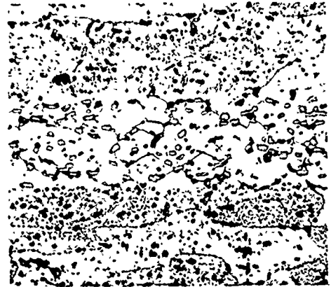
Mount #565 - Mag 250X 500 F - 25 Hours Boric Acid HF Etched
