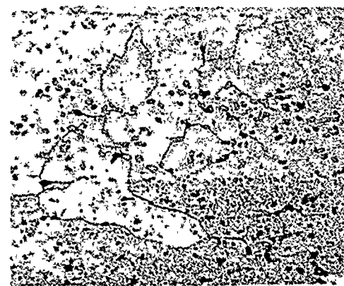
Bonding Cycle (24 PSI-60 Min.) Keller Etched - 250X - Mount #458
