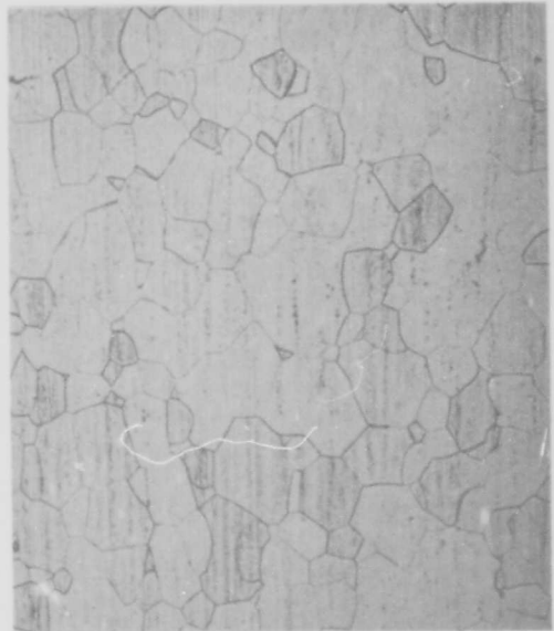
FIGURE 23 - Effect of Annealing on the Microstructure of Extruded Plus Swaged (92% R. A.) XB-88. 1 Hr. Anneals 100X
