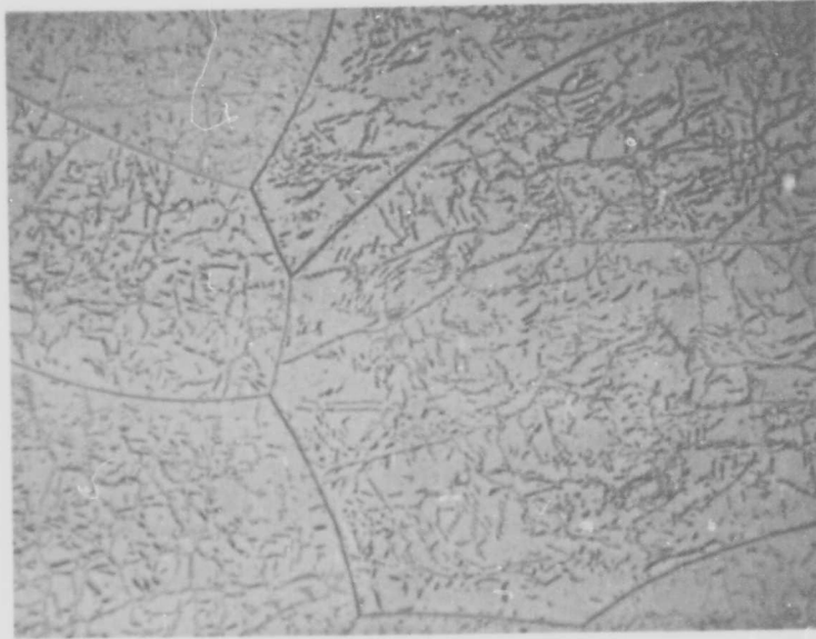
400X FIGURE 18 - Microstructure of XB-88 Annealed 2 Hrs. at 2000°C Plus 1 Hr. at 1600°C
