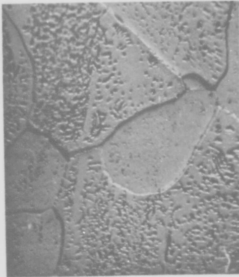
FIGURE 53 - Microstructure of XB-88 Creep Specimen (T-93) Annealed 1 Hr. at 1700^{\circ}\text{C} , Aged 88 Hrs. at 1315^{\circ}\text{C} . Failed after 117.6 Hrs. at 1315^{\circ}\text{C} ( 2400^{\circ}\text{F} ), 25,000 psi.
