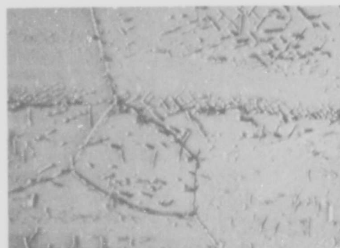
FIGURE 28 - Variation of Microstructure of Extruded Plus Swaged (92% R. A.) XB-88 with Annealing Time at 2200°C
