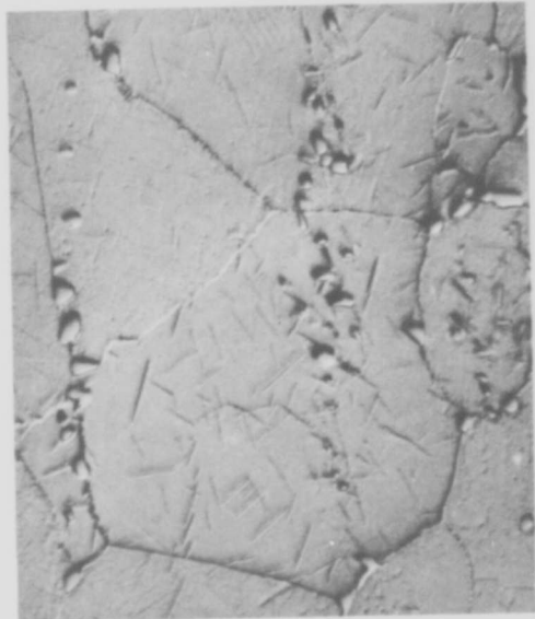
(a) Annealed 2 hrs. at 2000°C plus 1 hr. at 1800°C and Brine Quenched
