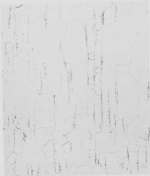
(b) Annealed 2 hrs. at 2000°C and Brine Quenched
