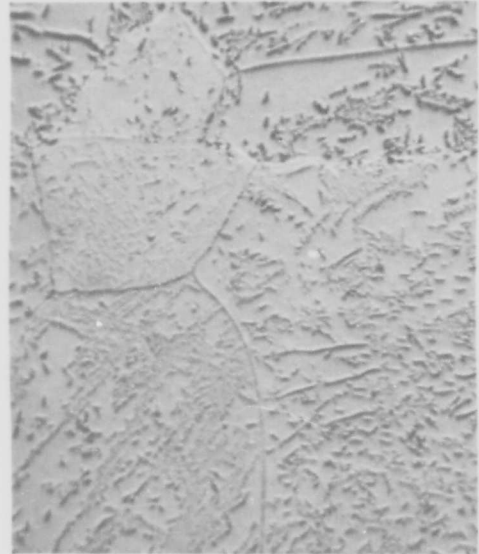
FIGURE 50 - Microstructure of XB-88 Creep Specimen Head Section. Dynapak Extruded at 1930^{\circ}\text{C} ( 3500^{\circ}\text{F} ). Failed After 41.7 Hours at 1315^{\circ}\text{C} ( 2400^{\circ}\text{F} ), 30,000 psi.
