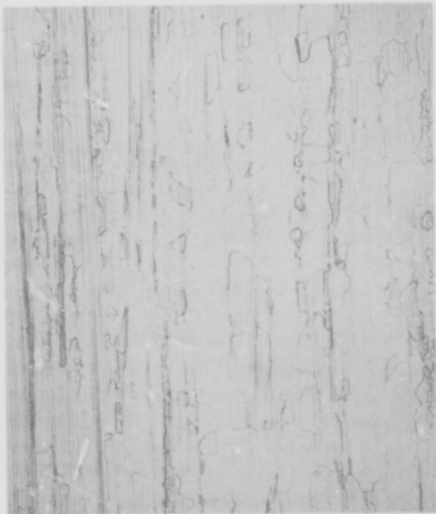
FIGURE 23 - Effect of Annealing on the Microstructure of Extruded Plus Swaged (92% R. A.) XB-88. 1 Hr. Anneals 100X
