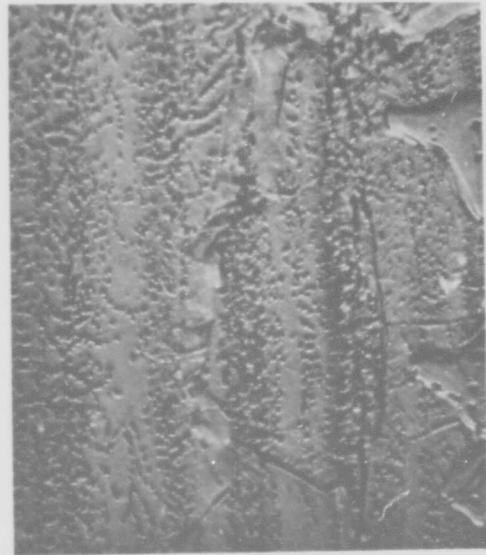
FIGURE 53 - Microstructure of XB-88 Creep Specimen (T-93) Annealed 1 Hr. at 1700^{\circ}\text{C} , Aged 88 Hrs. at 1315^{\circ}\text{C} . Failed after 117.6 Hrs. at 1315^{\circ}\text{C} ( 2400^{\circ}\text{F} ), 25,000 psi.
