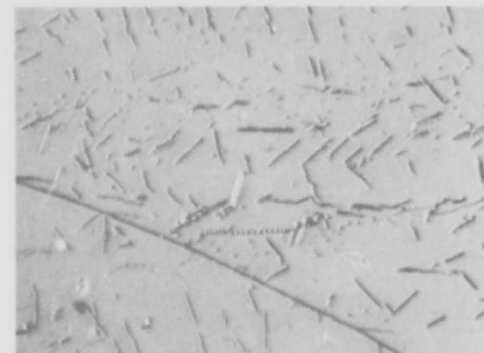
FIGURE 28 - Variation of Microstructure of Extruded Plus Swaged (92% R. A.) XB-88 with Annealing Time at 2200°C
