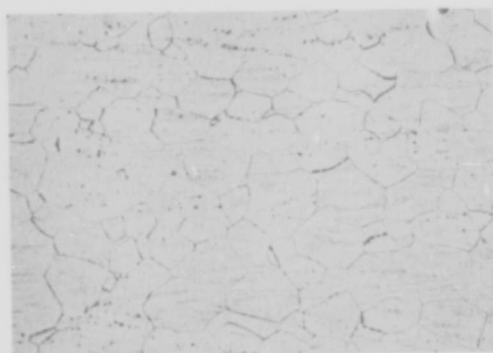
FIGURE 27 - Variation of Microstructure of Extruded Plus Swaged XB-88 as a Function of Annealing Time at 1800°C
