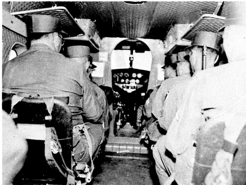
Fig. 14. View looking forward in the cabin, showing the seating arrangement utilized in transporting combat troops.
