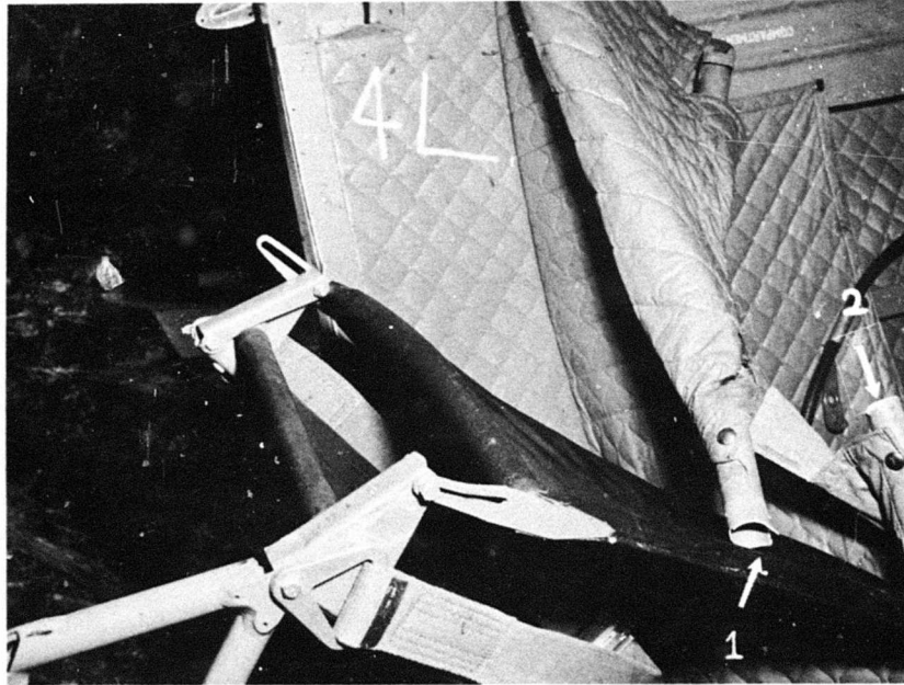
Fig. 43. Failure of the luggage compartment post utilized as one of the seat attachments is shown by arrows 1 and 2.
