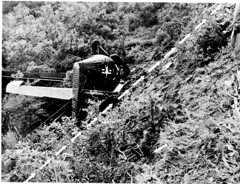
Fig. 6. The side slope of the terrain at the point of principal impact with the ground was approximately 40 degrees. Analysis indicates that the left wing of the aircraft was down about 60 degrees when the wing tip first struck the ground; this resulted in a 20-degree wing-down angle with relation to the terrain at the instant of impact. Note the gouge (arrow) caused by the left landing gear.
