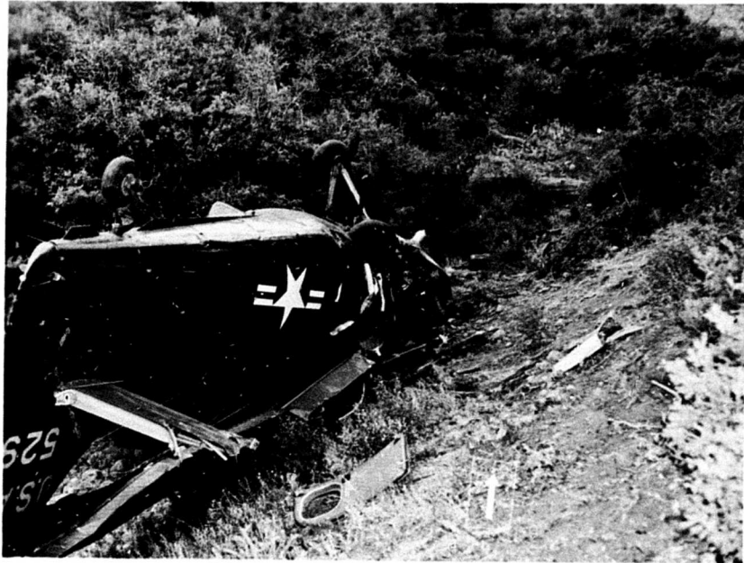
Fig. 5. View showing gouging (arrow) caused by the aircraft's decelerating along the ground following the principal impact. Note the relative intactness of the rear cabin and fuselage structure.
