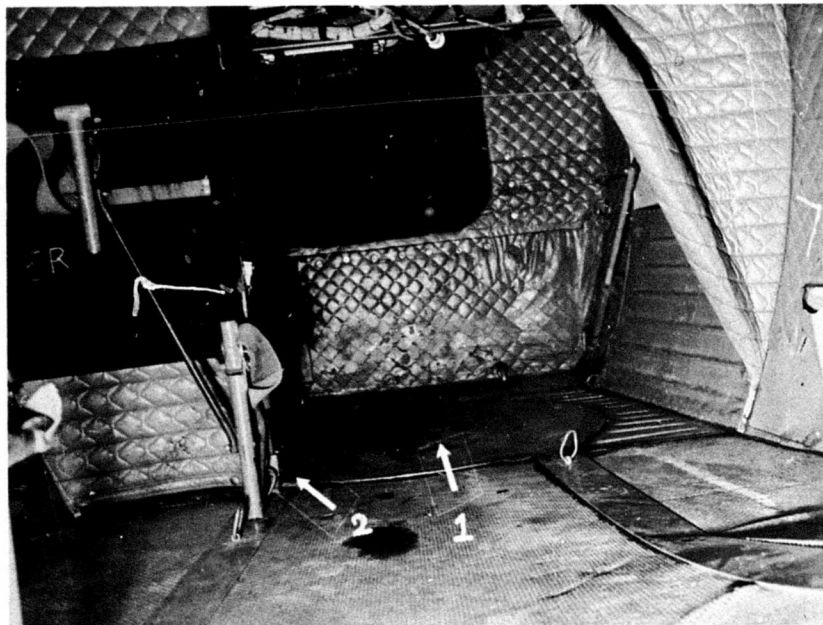
Fig. 26. View of the right-rear cabin area. A toolbox that was carried unsecured on the luggage compartment floor (arrow 1) was found rammed against the left vertical support of seat 5R (arrow 2), and impaled on two exposed bolt ends. It remained attached to them as the aircraft rolled to a partially inverted attitude during the crash sequence.
