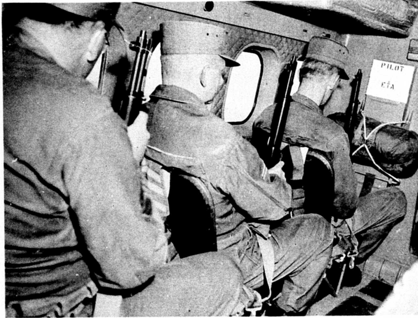
Fig. 15. View of the left-hand cabin area, showing the manner in which combat troops position their weapons during flight. (Passenger occupying the rearmost seat is not shown.)
