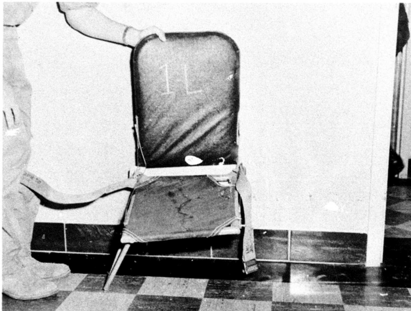
Fig. 44. Seat 1L remained completely intact and in its normal position in the cabin during the crash. However, both aisle floor attachments were distorted, and the safety belt revealed evidence of incipient failure at its anchorages to the seat pan.
