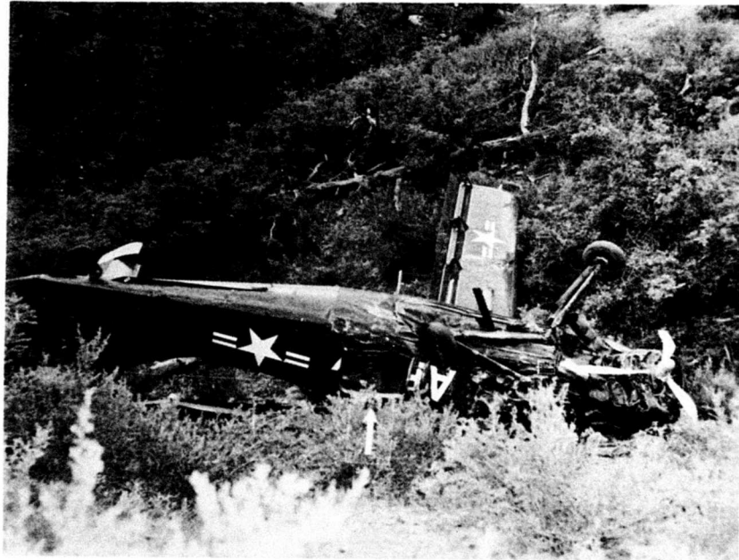
Fig. 7. View showing overall damage to the underside of the fuselage, landing gear, and nose structure. The main cabin door was torn free during the crash, and the open doorway (arrow) was subsequently utilized for evacuation by the cabin passengers.
