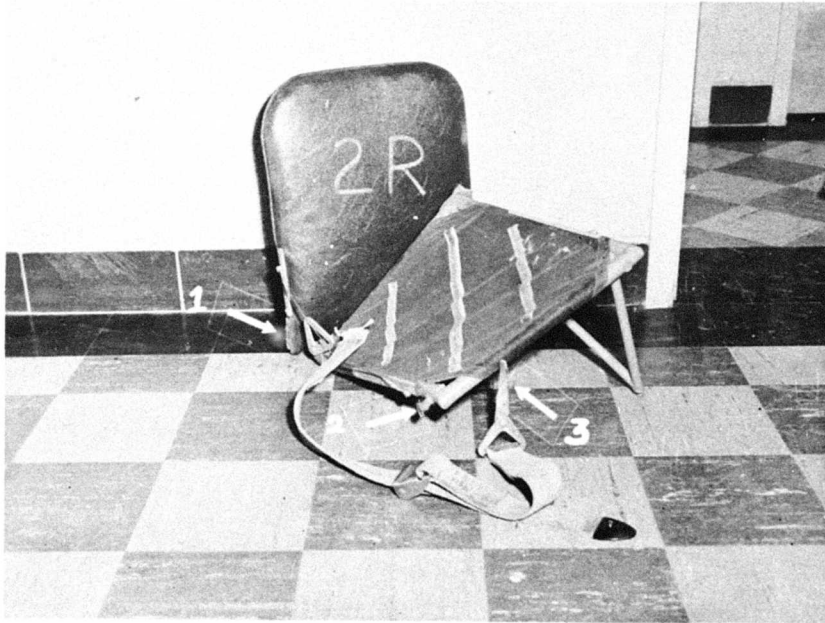
Fig. 49. Seat 2R was severely damaged during the crash. The seat back was torn free from the seat pan because both of the metal straps joining and hinging the back to the pan (arrow 1) failed. Both aisle floor anchorages and the rear wall anchorage tore completely free; the forward wall fitting was badly distorted (arrow 2).
