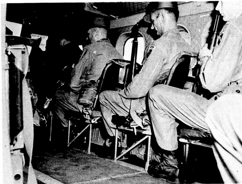
Fig. 16. View of the right-hand cabin area, showing the seating configuration utilized in transporting combat troops. (Note positioning of weapons, with muzzle near face and head.)
