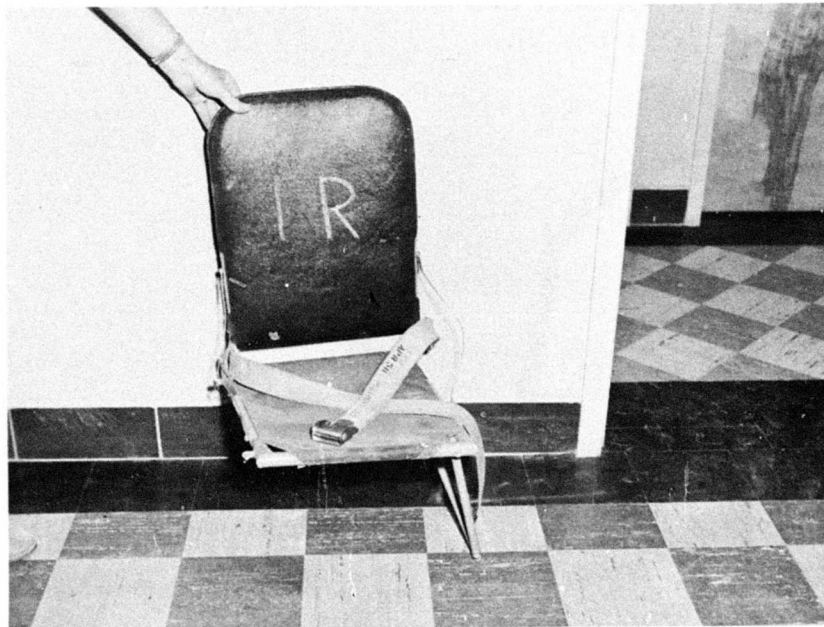
Fig. 48. Seat 1R was the only seat in which the safety belt, seat pan, seat back, and all seat anchorages remained completely intact. The occupant of this seat, who was restrained by his seat belt, received moderate injuries that were apparently caused by his striking his head and upper torso against the bulkhead separating the cockpit and the cabin.
