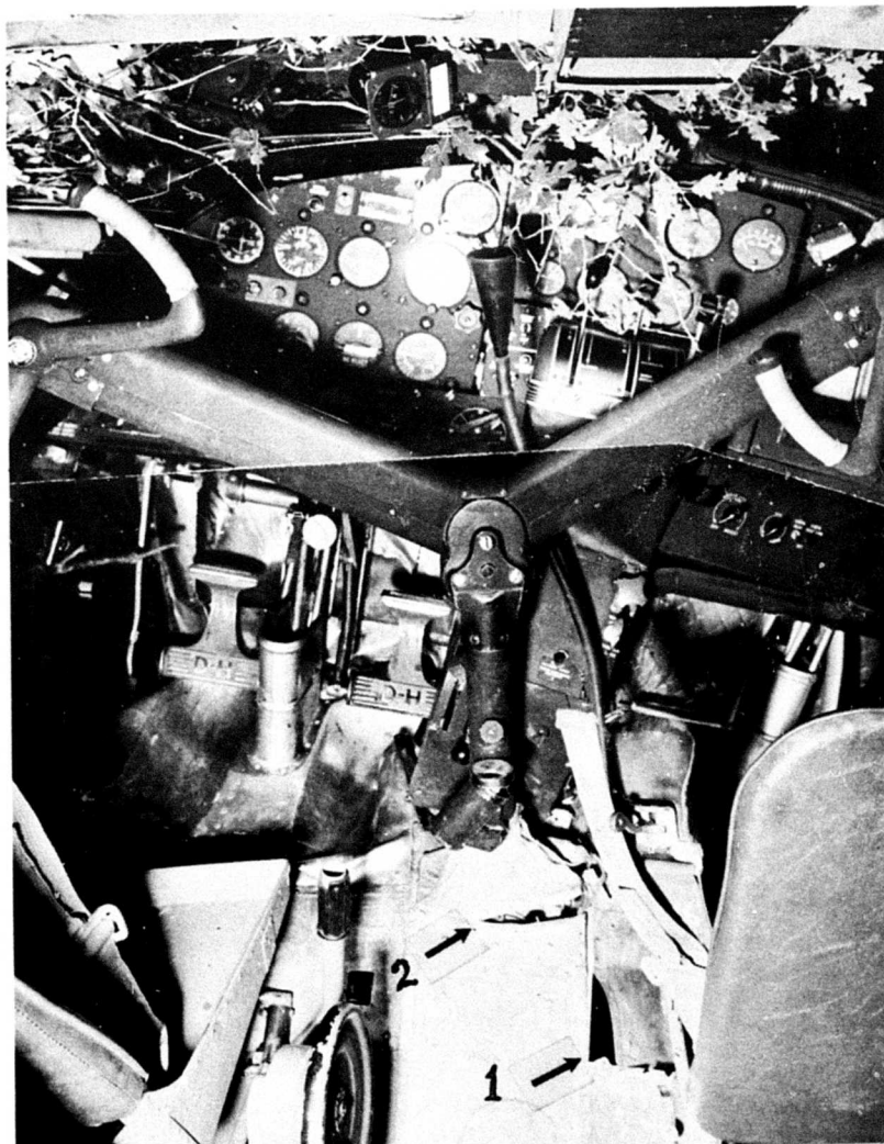
Fig. 17. Interior view (composite photo) of "intact" cockpit area. The upheaval and collapse of the floor structure (arrow 1) and the tearing free of the control column (arrow 2) probably occurred at the principal impact.
