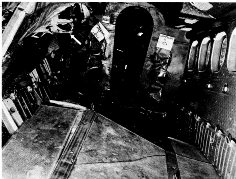
Fig. 28. Looking forward in the cabin after removal of the passenger seats. Note the upward displacement of the cabin floor and the inward displacement of the left cabin wall and ceiling structure in the vicinity of the wing root (arrow).
