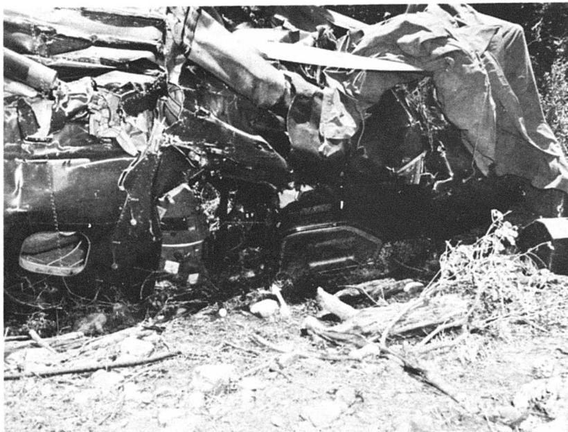
Fig. 11. The cockpit doorway (arrow), although "popped" open during the crash, was not available as an emergency exit because the aircraft was resting partially on its left side. The pilot and copilot escaped through the broken front windshield.
