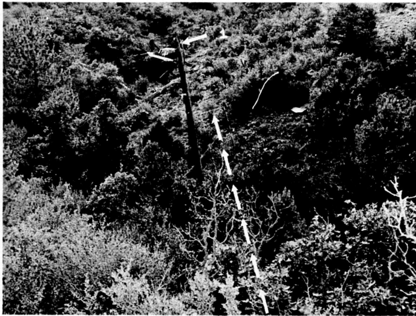
Fig. 3. View looking forward along flight path (indicated by line of arrows) showing final resting place of the aircraft. The dead tree (arrow 1) was struck by the leading edge and underside of the left horizontal stabilizer at a point approximately 6 feet above the present top of the tree trunk.
