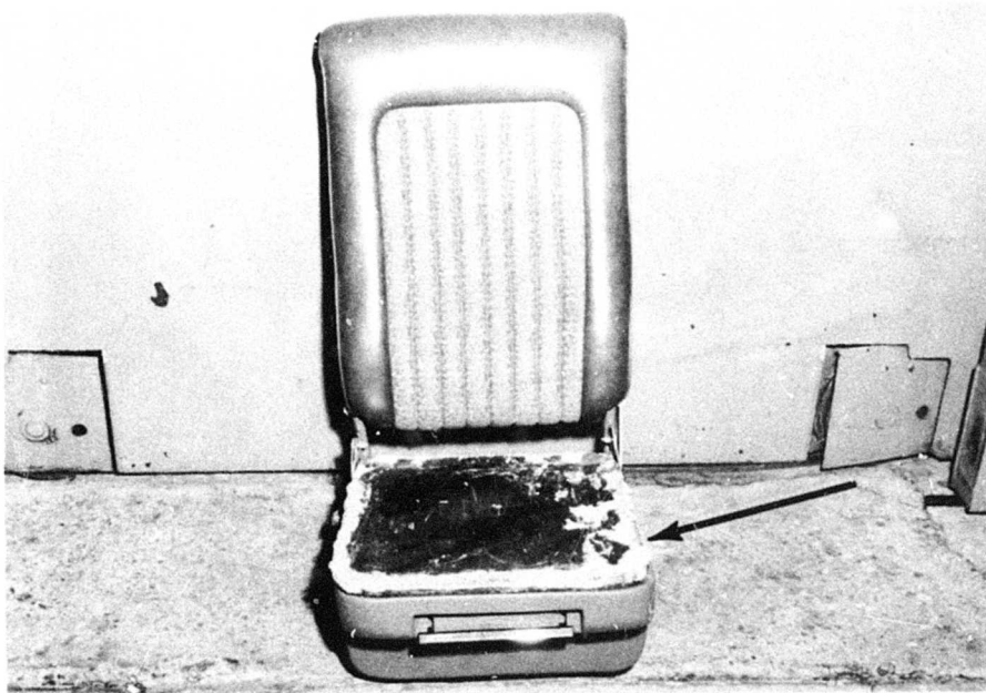
Fig. 61. Polyurathane cushion, cemented to the neoprene-impregnated nylon seat pan, is removed. The seat pan does not appear to have any degree of yield or stretch.
