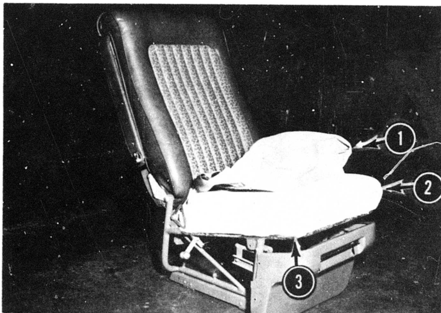
Fig. 59. Plastic (leatherette) upholstery (arrow 1) was removed from the seat cushion, revealing a 4-inch thick cushion of foamed polyurathane (arrow 2). This cushion was cemented to the top of the seat pan (arrow 3).
