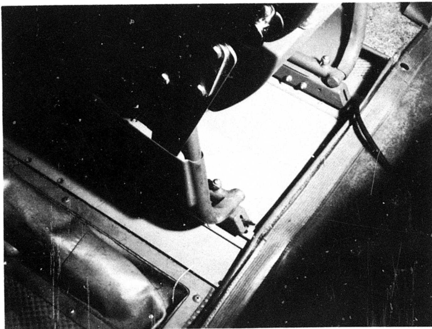
Fig. 57. Seat tracks on mounting plate afford fore/aft adjustment.
