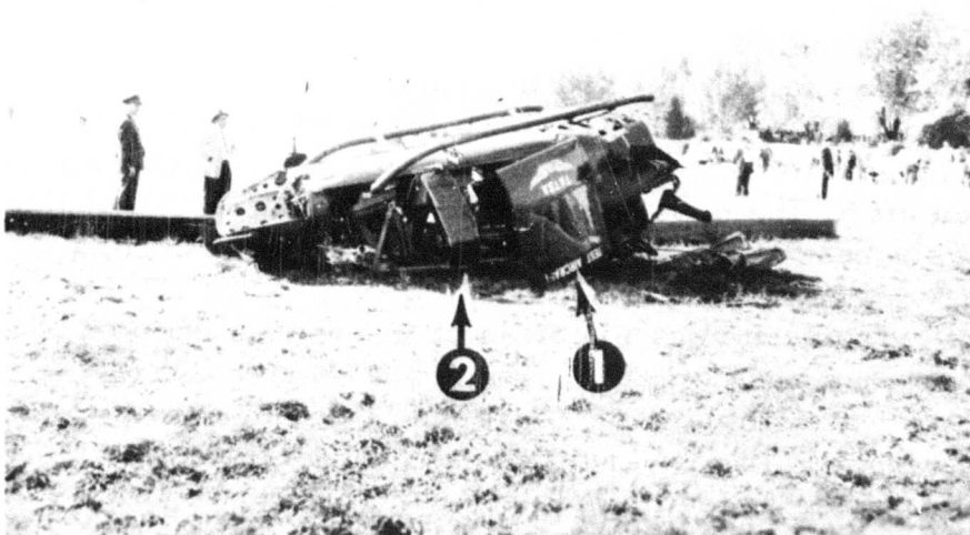
Fig. 65. Right side of helicopter. Cargo door (arrow 1) was out of its track, but still attached to the fuselage. Note inward deformation of "roof" structure and buckling of vertical support member (arrow 2).
