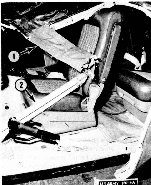
Fig. 22. Instrument panel broke forward (away from occupants) during crash (arrow).
