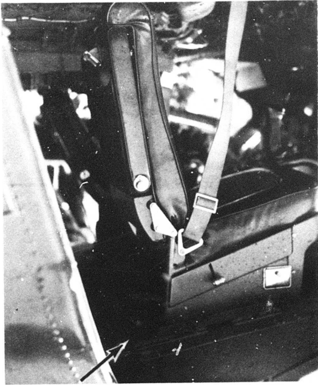
Fig. 56. Pilot's seat is shown installed in the HU-1A. Mounting plate, upon which seat tracks were mounted, was held to aircraft floor with 16 bolts.
