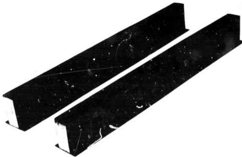
Figure 79. "Thornel" 40/ERL 2256 Beams with Balsa Wood Cored.
