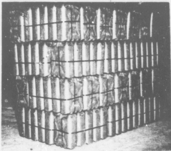
Figure 20. Bundled plastic containers stacked upright in a straight stack, four layers with ten 5-container bundles per layer.
