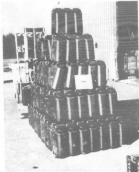
Figure 9. Empty loose steel containers in alternating vertical and horizontal layers.
