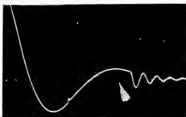
b) Derivative of magnetic field, B , at surface of sand. Vertical Scale = 50 mV/cm
