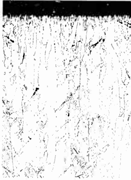
Figure 22. 200X Photomicrograph of Vapor-Deposited Tungsten Crucible after 30 Minutes Operation with Fuel Byproducts at 1700°C. No Evidence of Attack.
