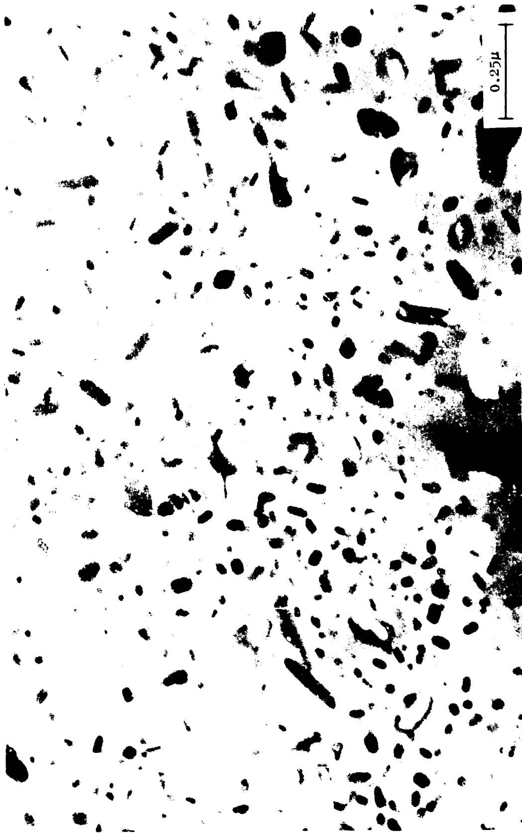
Figure 5. Micrograph of 7075-T6 Specimen After Over-Aging for 210 Hours at 350 F
