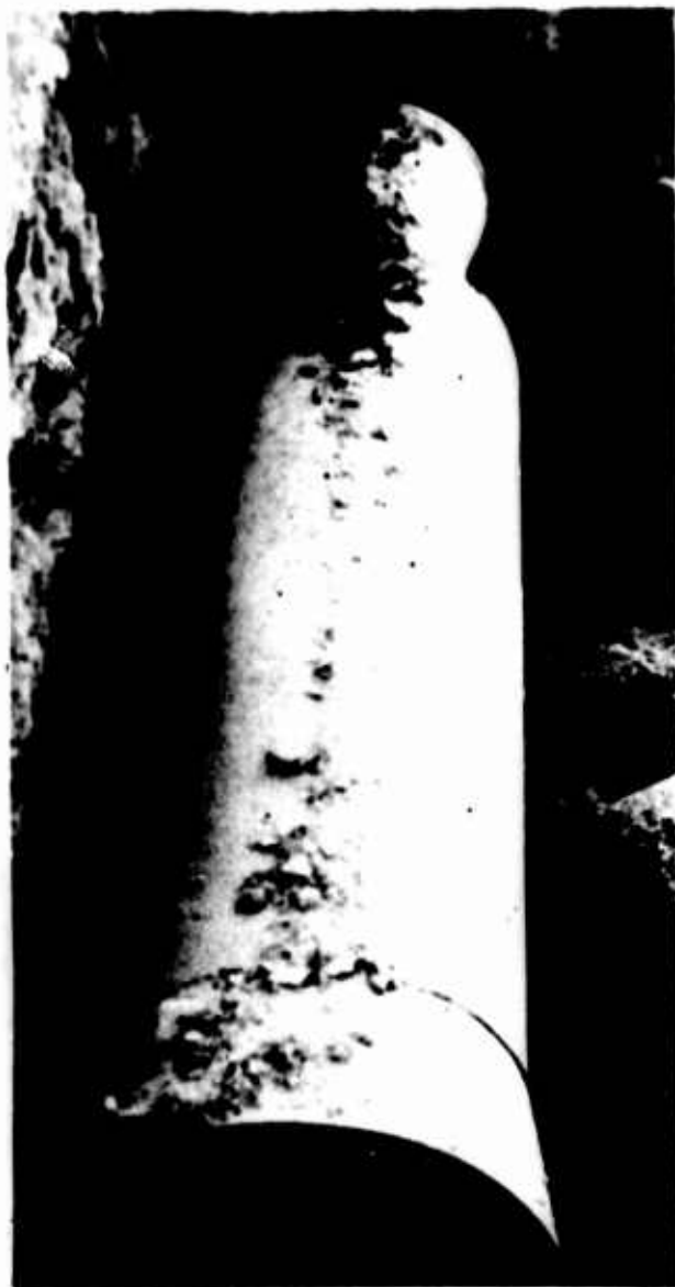
FIGURE 18: THE REMAINS OF THE ROCKET MOTOR AFTER INITIATION OF THE DETONATING CORD. (TEST 4)
