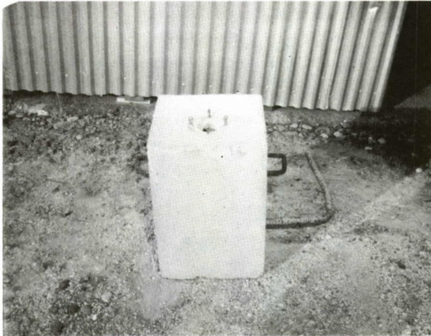
Figure 21. Surface Air-Pressure Transducer Mount
