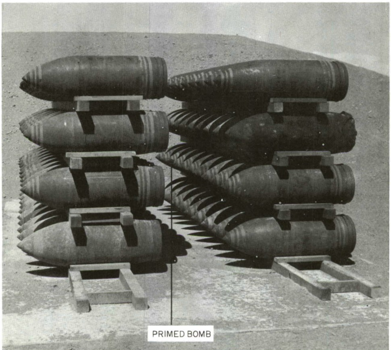
Figure 16. Phase IV Donor Stack Showing the Single Primed Bomb
