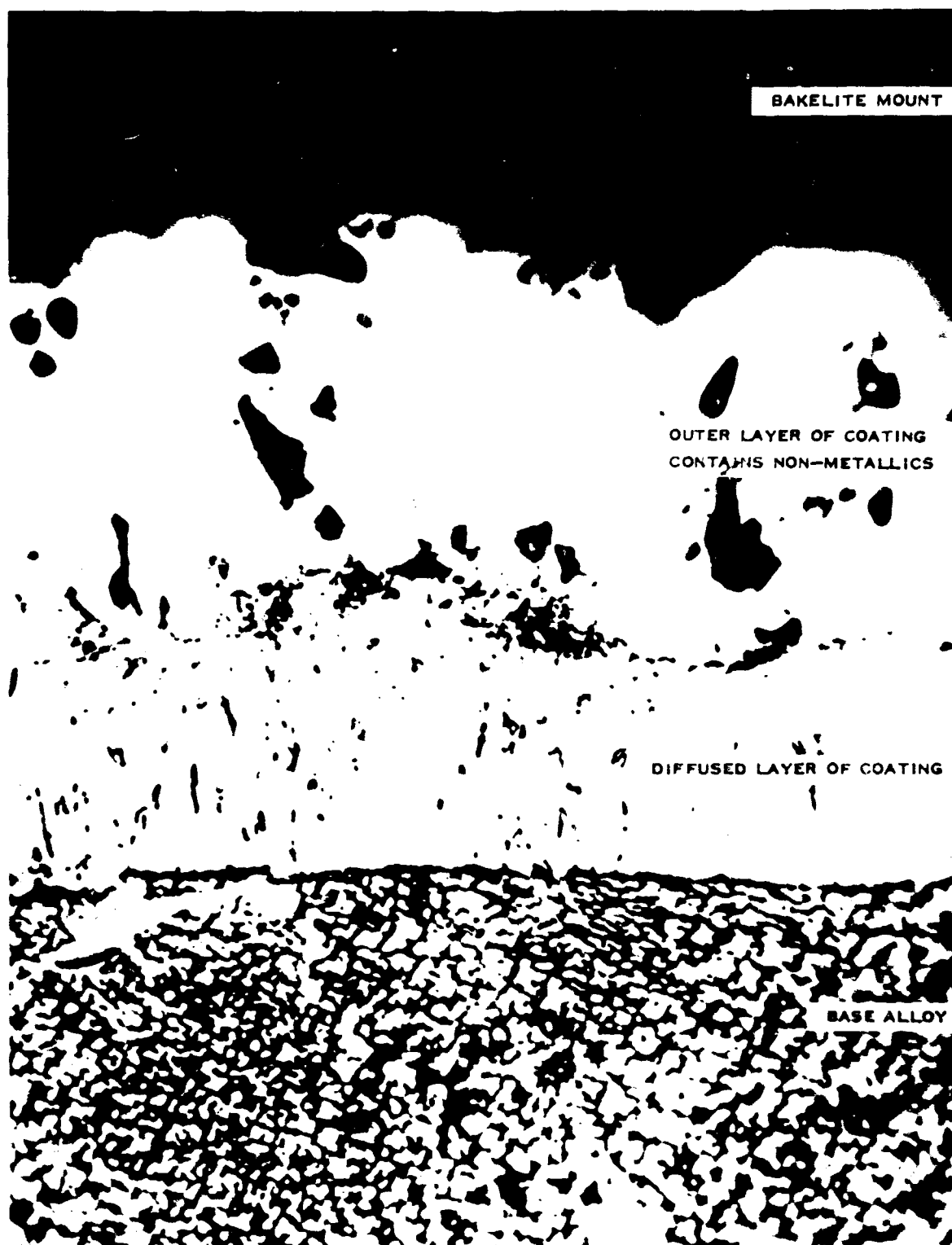
METALLOGRAPHIC CROSS-SECTION. 3% SULFURIC ACID-ELECTROLYTIC ETCHED. 2000X MAGNIFICATION.
