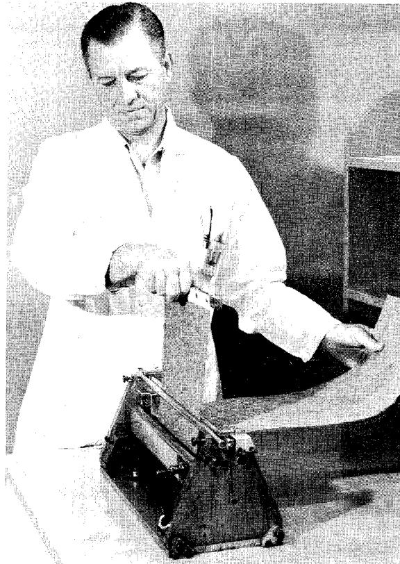
Figure 4. Technician Impregnating Amercoat C10-G15 Crocidolite Asbestos Mat with Skybond 700 Polyimide Resin Using Laboratory Dip Tank Coater
