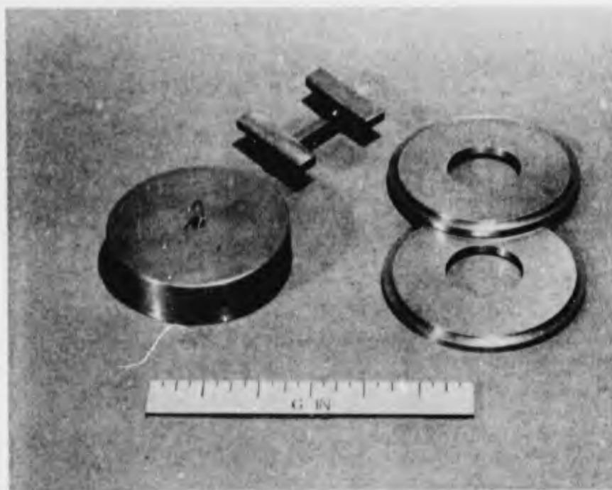
FIGURE 56. WEIGHTS AND WEIGHT PLATFORM USED FOR CREEP TESTING BORON FILAMENTS
