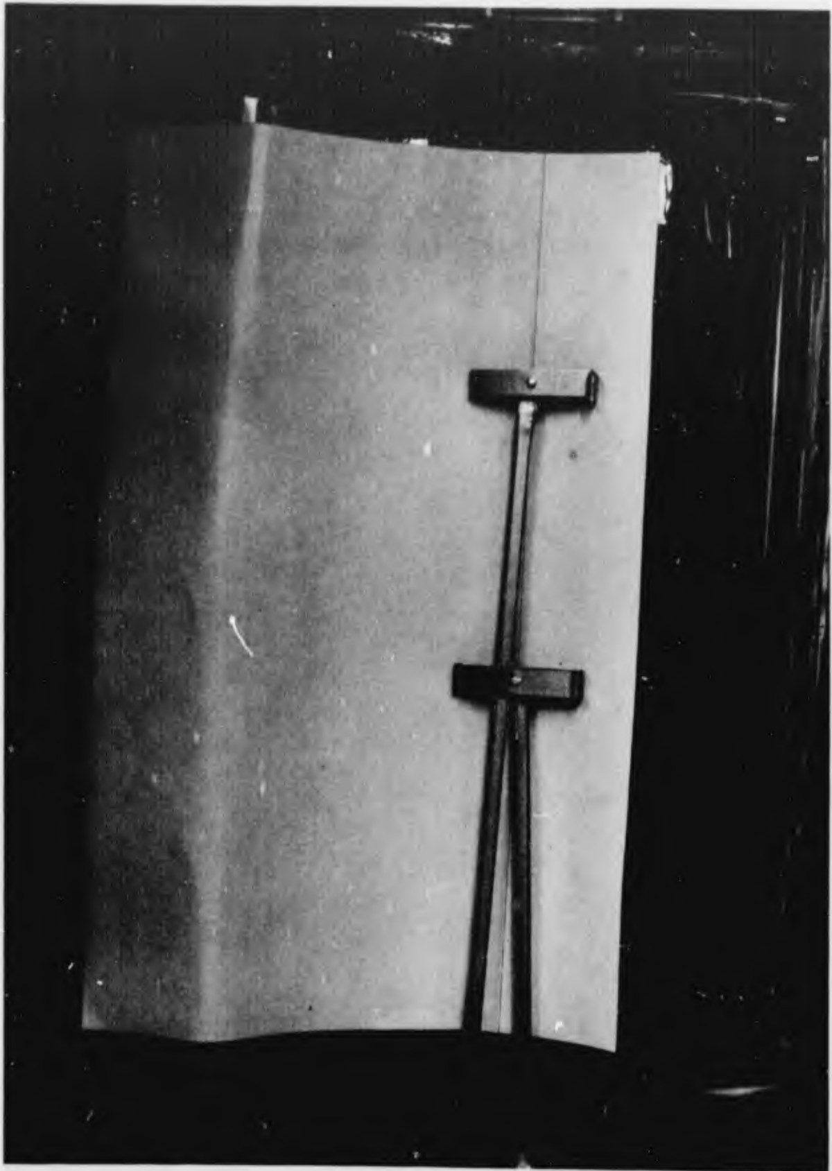
FIGURE 58. CLIPS AND PUSHRODS OF DOUBLE BEAM EXTENSOMETER ATTACHED TO BORON FILAMENT
