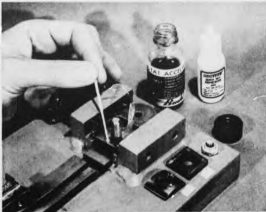
A. Applying Adhesive to Position Filament in Grip
