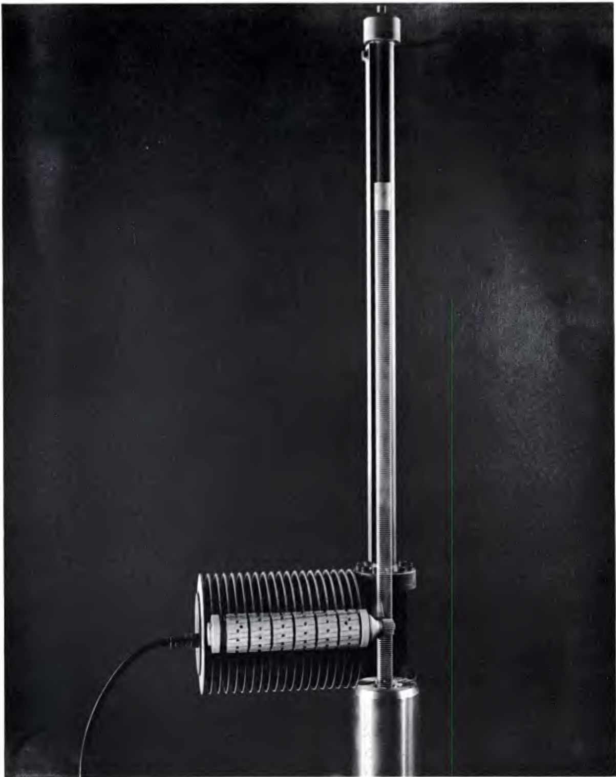
Fig. 3.15--Phantom view of Marvel-Schebler control rod drive
