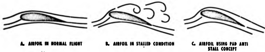
Figure 1. Emergency Control of Boundary Layer on Airfoil Wing by Propellant Energy
