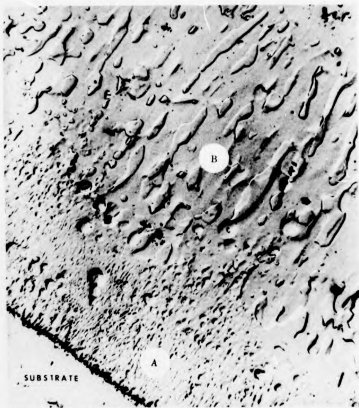
Figure 121. Electron Micrograph of As-Applied Phase VII Sylvania SiCrTi Slurry Coating on XB-88 Alloy Showing Columnar Growth Within the Diffusion Zone (A) and Intermediate Coating Layer (B)
