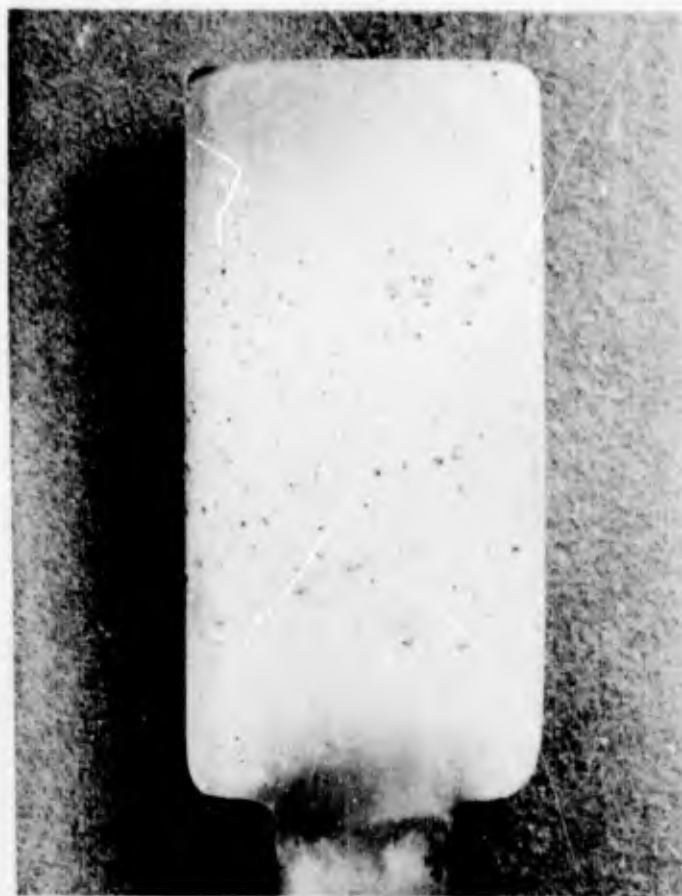
Figure 109. Convex Airfoil Surface of Modified TRW TiCr-Si (Vacuum) Pack Coated XB-88 Alloy Specimen Showing Spot Oxidation Failures After Thermal Fatigue Testing for 600 Cycles to 2200°F
