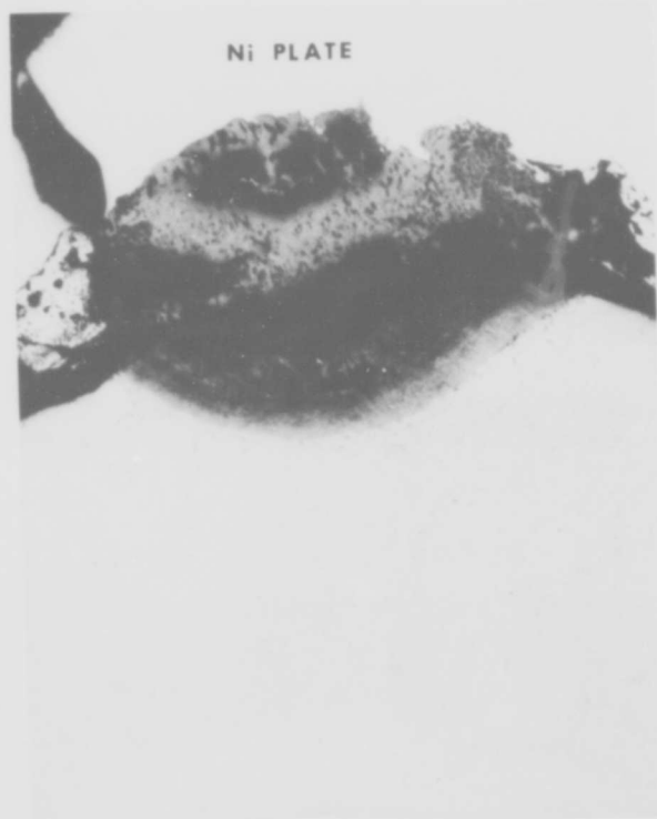
Figure 50. Microstructure of Solar MoTi-Si Coated Cb-132M Alloy Showing Substrate Oxidation Beneath Bisque-Colored Glassy Areas After Oxidation-Erosion Testing
