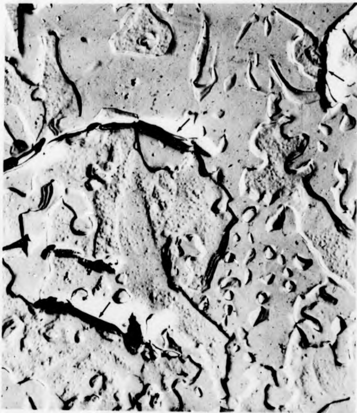
Figure 123. Electron Micrograph of As-Applied Phase VII Sylvania SiCrTi Slurry Coating on XB-88 Alloy Showing Lateral Microcracks (Arrows) and the Absence of Diffusion Surrounding Precipitated Particles in the Outer Coating Region
