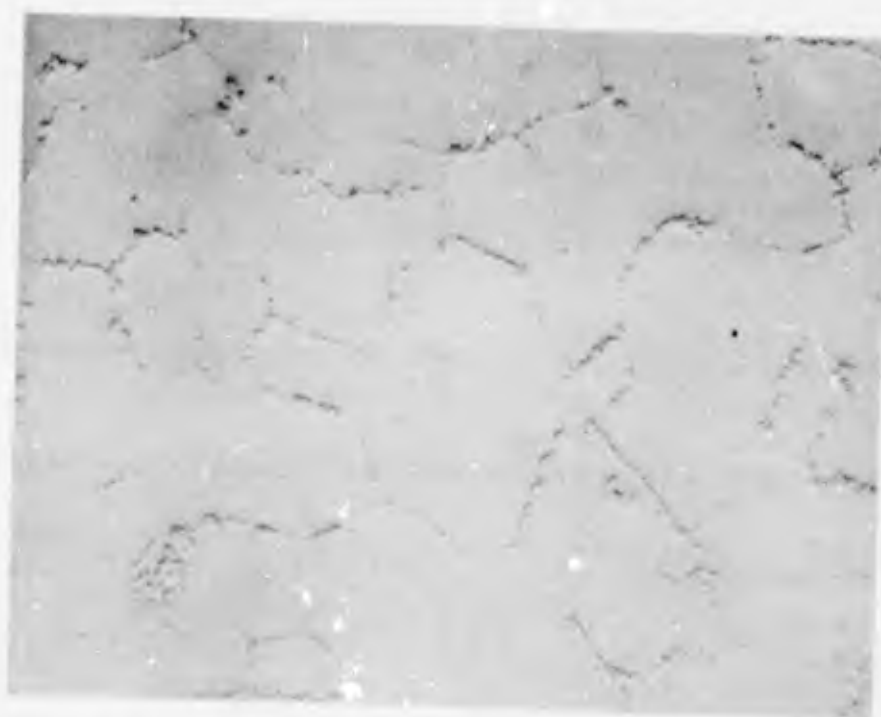
Figure 44. Microstructure of Cb-132M Alloy Substrate Showing Grain Boundary Oxygen Enrichment Beneath a Typical Solar V-CrTi-Si Coating Failure in 2200°F Oxidation-Erosion
