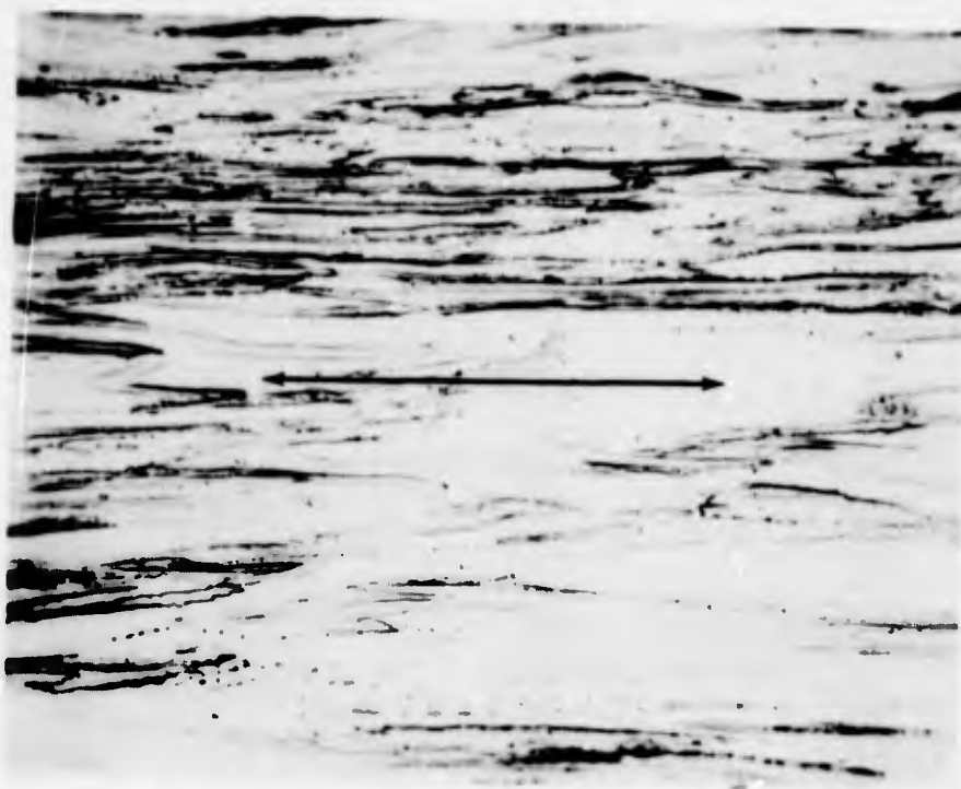
ALLOY: XB-88, SWAGED BAR PLANE: PARALLEL TO BAR AXIS (ARROW) ETCH: 33% HYDROFLUORIC ACID, 33% NITRIC ACID, 33% WATER MAG: 500X
