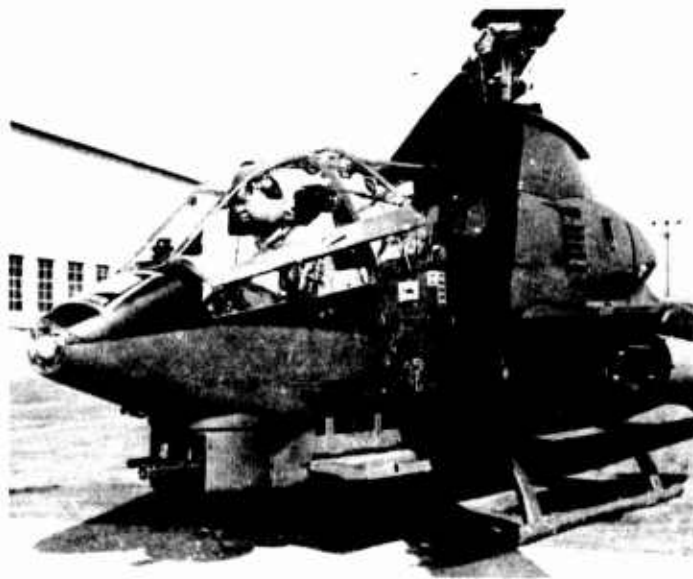
PHOTO 2 - AH-1G helicopter, depicting stow area for ammunition cans in side compartment and the oscillograph installation in wing pod .
