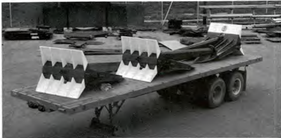
Figure 8. 6,000-pound STATO anchors with stabilizers folded to facilitate truck shipment.
