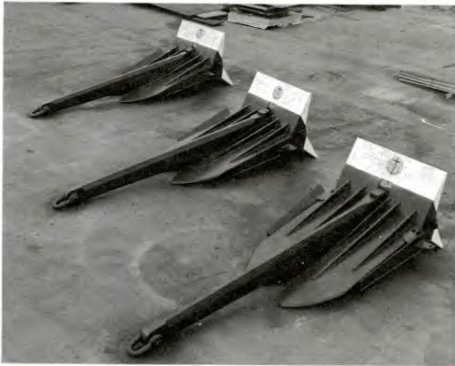
Figure 12. STATO (6,000 pound) anchors with hinged stabilizers.
