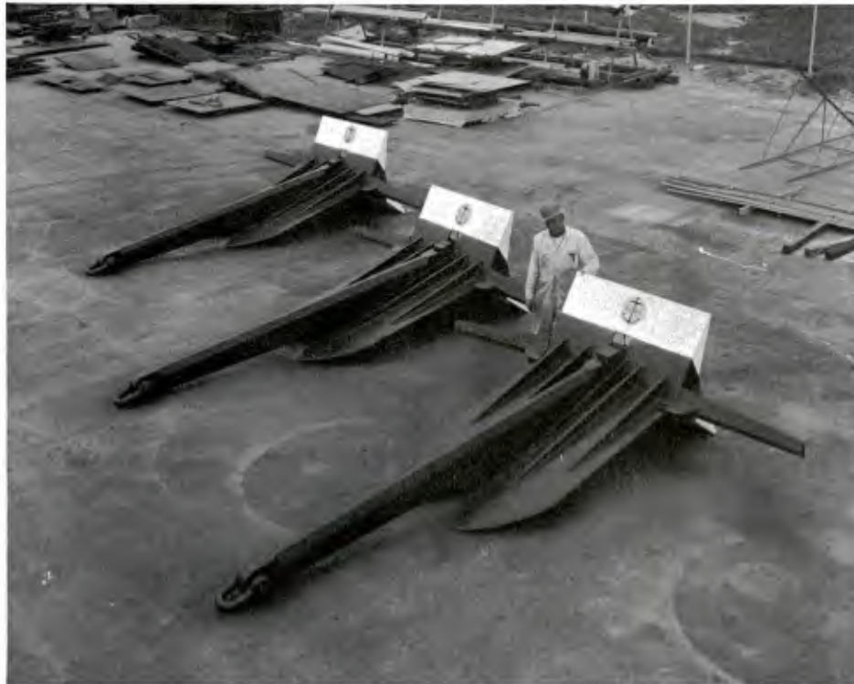
Figure 6. 6,000-pound STATO anchor. The light portion under man's hand is a palm extension plate for mud operation.
