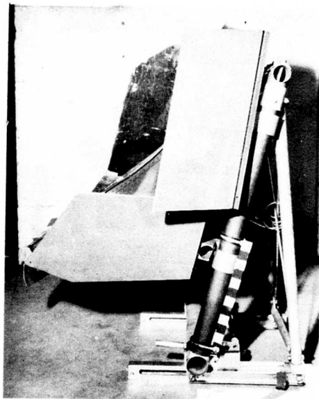
Figure 5. Side View - Hayes Armored Aircrew Survival Seat.
