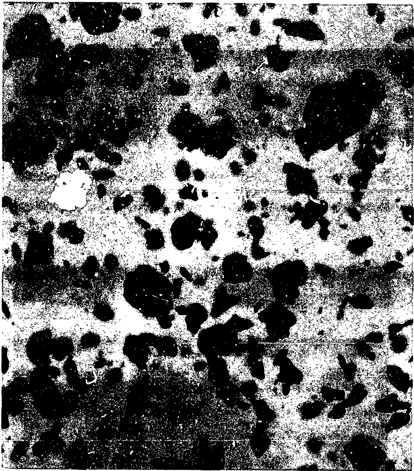
Figure 3. Optical Micrograph of Sample 243-123-2 - Flaked Zn-dust Average Flake Thickness = 2.5\mu Magnification = 1,000X
