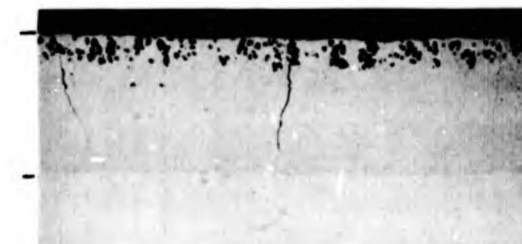
Figure 104 Microstructures of V-CrTi-Si Coated Columbium Alloys after a 4 hour Low Pressure (0.1-0.5mm) Exposure at 2400°F. 250X
