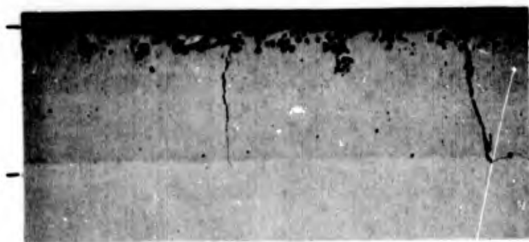
Figure 103 Microstructures of V-CrTi-Si Coated Columbian Alloys after a 4 hour Low-Pressure (1-5 mm) Exposure at 2400°F. 250X
