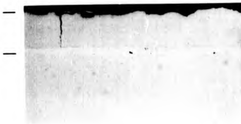
Figure 48 Microstructures of Mo-CrTi and Mo-CrTi-Si Coated Cb-752. 250 X
