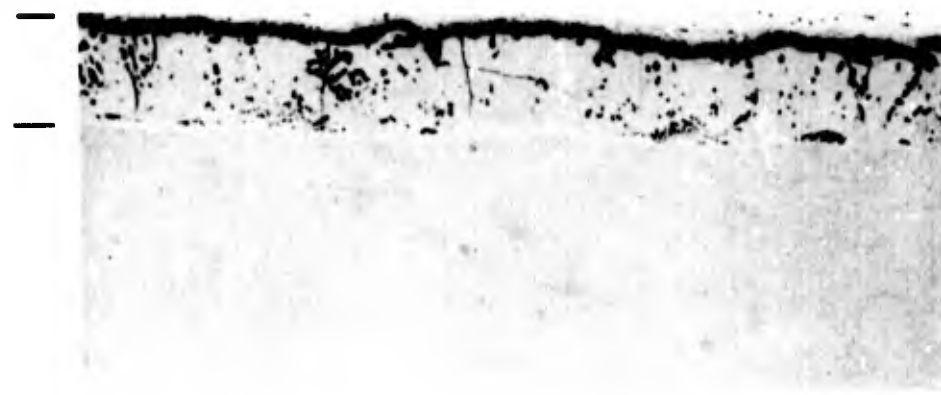
Figure 19 Microstructures of Silicide Coating Systems on Cb-752 Alloy. Run Numbers in Parenthesis 250 X
