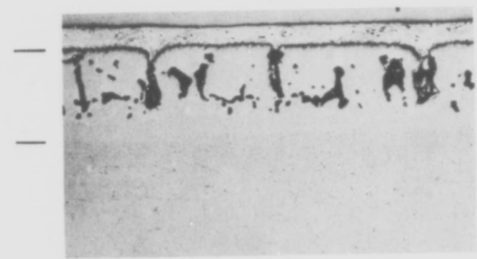
Figure 41 Microstructures of Columbian Alloy Cb-752 after V, Al and Cr-Ti Coating. 100 X
