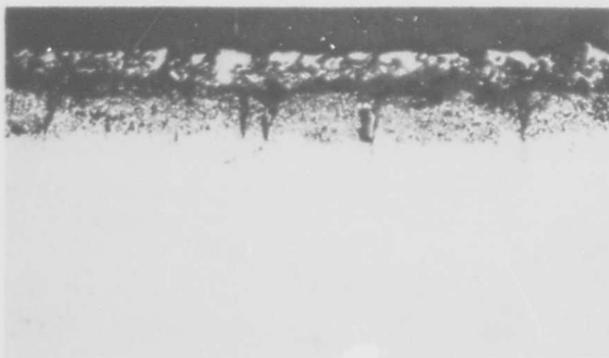
Figure 43 Photomicrographs of Phase II Exposed V-Al-CrTi-Si System Coatings on Cb-752. 100 X
