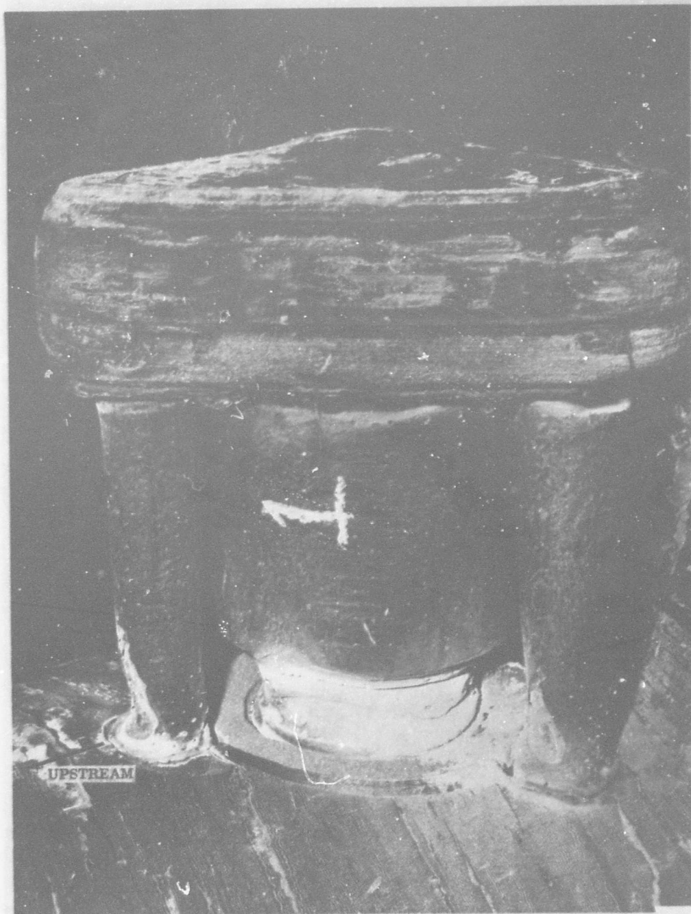
Figure 12. Valve and Orifice 1 After Test
