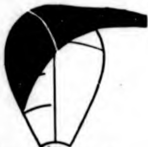
Figure 13 - Back Cavitation at an Advance Coefficient of 0.77
