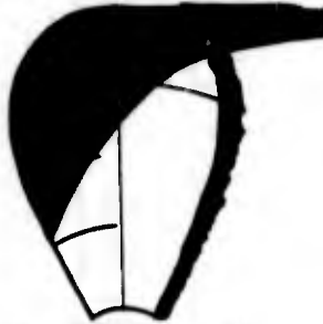
Figure 13 - Back Cavitation at an Advance Coefficient of 0.77
