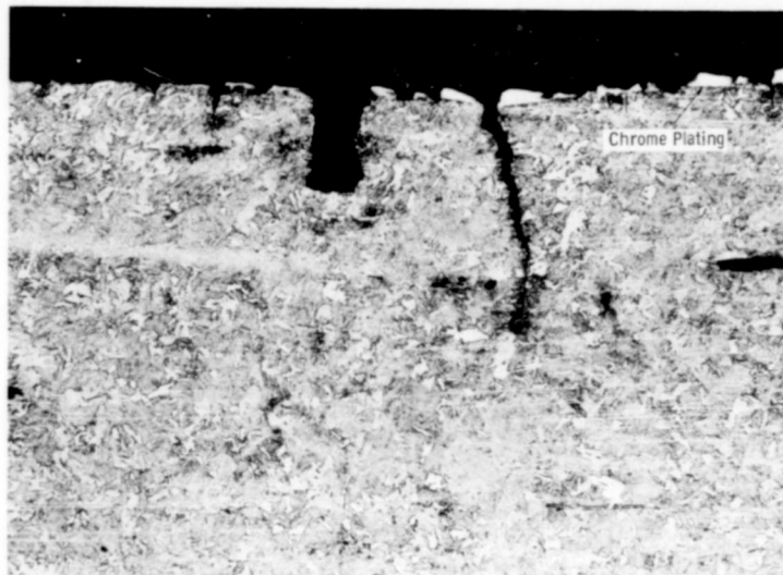
Figure 4. Cross Section of Inside of Chrome Plated .257 cal Gun Barrel Near Cartridge Seat, After 1200 Rounds - Transversal, 100x
