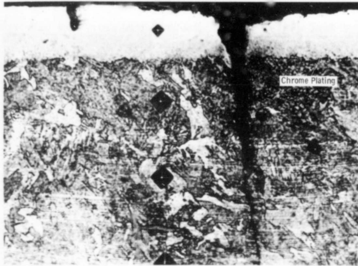
Figure 5. Cross Section of Inside of Chrome Plated .257 cal Gun Barrel near Cartridge Seat, After 1200 Rounds - Longitudinal, 500x
