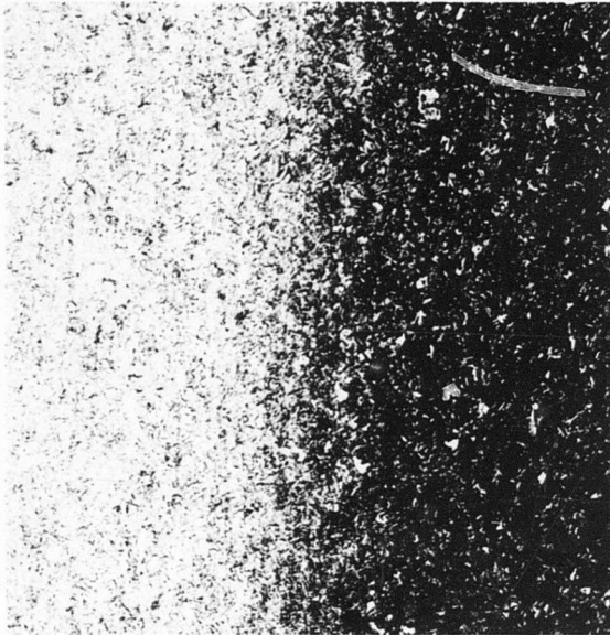
Extrusion No. 2 - 2-1/2" I.D. (Acceptable Bond)
