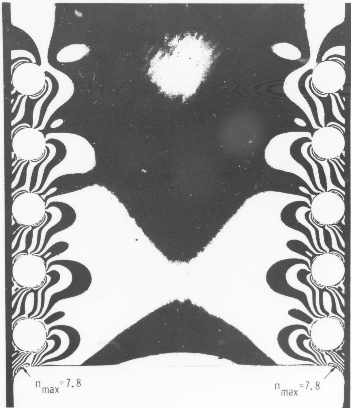
Fig. 3 ISOCHROMATICS IN A RECTANGULAR PLATE WITH A SERIES OF CIRCULAR PERFORATIONS, BONDED ALONG ITS SIDES, AND SUBJECTED TO RESTRAINED SHRINKAGE
