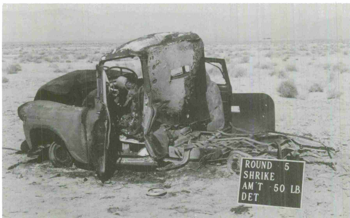
FIG. 18. Condition of Truck After Detonation of 50 Pounds of PBXC-104 Explosive, Test 5.
