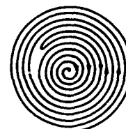
45 in OD, 0.5 in ID, 28 turns (inner turns opposite direction)
