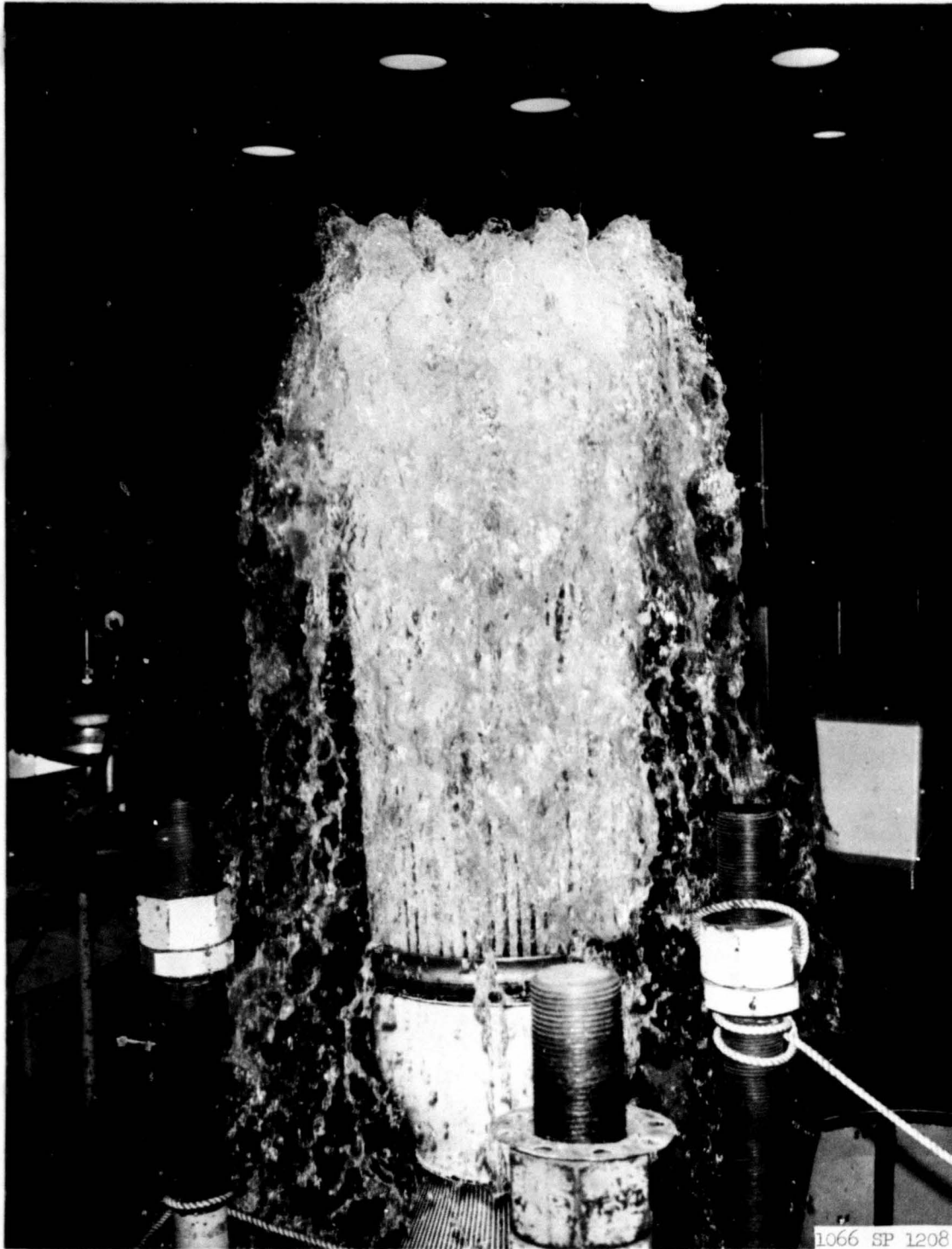
Figure 37 -- Combustion Chamber Flow Test to Atmosphere
