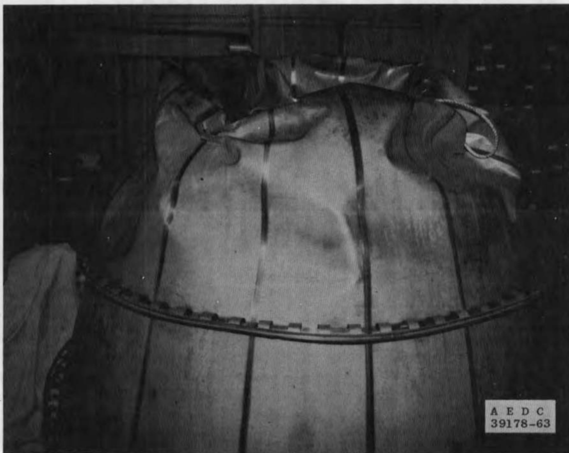
Fig. 6 Nozzle Extension Failure during Test B-2, Configuration I
