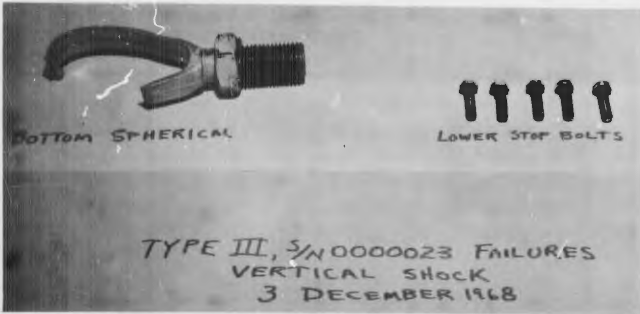
Figure 15. Type III, S/N 23, Test Failures
