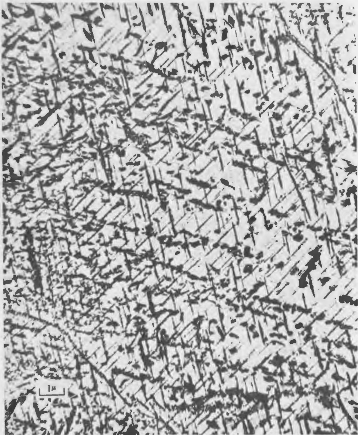
FIGURE 36. TEM of (111) Foil of B-88 (Specimen A-1) Creep Tested 168 Hours at 2200 F, 34,000 psi into 3rd Stage Creep. Plastic Strain = 1.66%.
