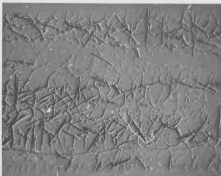
FIGURE 49. Microstructure of VAM-98 (Cb-22W-2Hf-0.05C-0.04N) Solution annealed 1 hour at 1800°C and helium cooled plus aged 7 hours at 1100°C.
