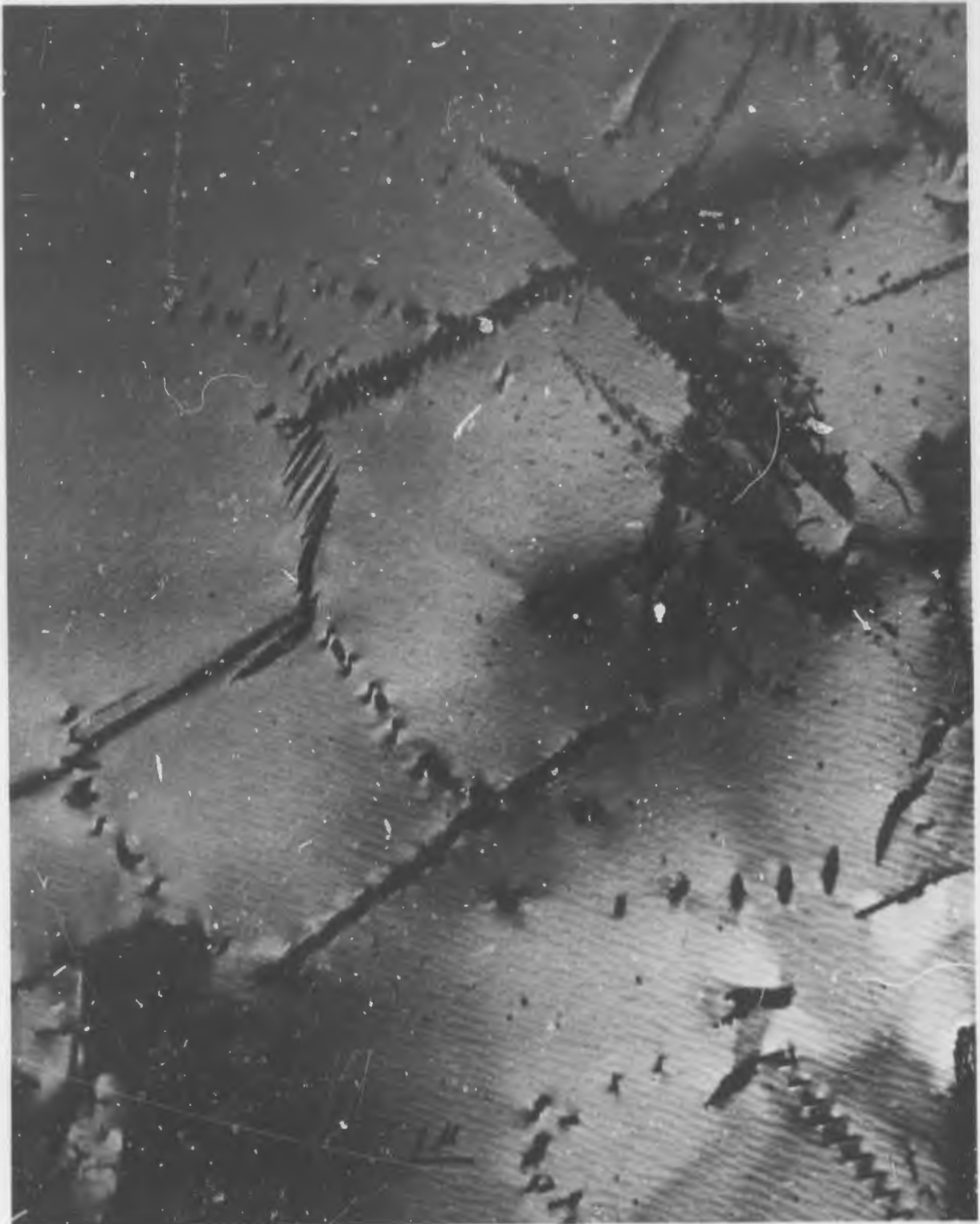
FIGURE 57. Transmission Electron Micrograph of VAM-98 (Cb-22W-2Hf-0.05C-0.04N) Solution annealed 1 hour at 1800°C and helium cooled; plus aged 7 hours at 1100°C. Thin foil showing general precipitation formed substructure.
