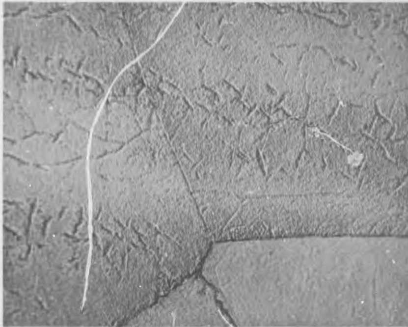
FIGURE 51. Microstructure of VAM-98 (Cb-22W-2Hf-0.05C-0.04N) Solution annealed 1 hour at 1800°C and helium cooled plus aged 12 hours at 1100°C.
