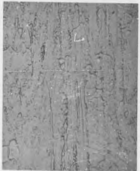
FIGURE 3 - Effect of Annealing on the Microstructure of Cb-1 Processed by G. E. Sequence 1 Hour Anneals. 400X
