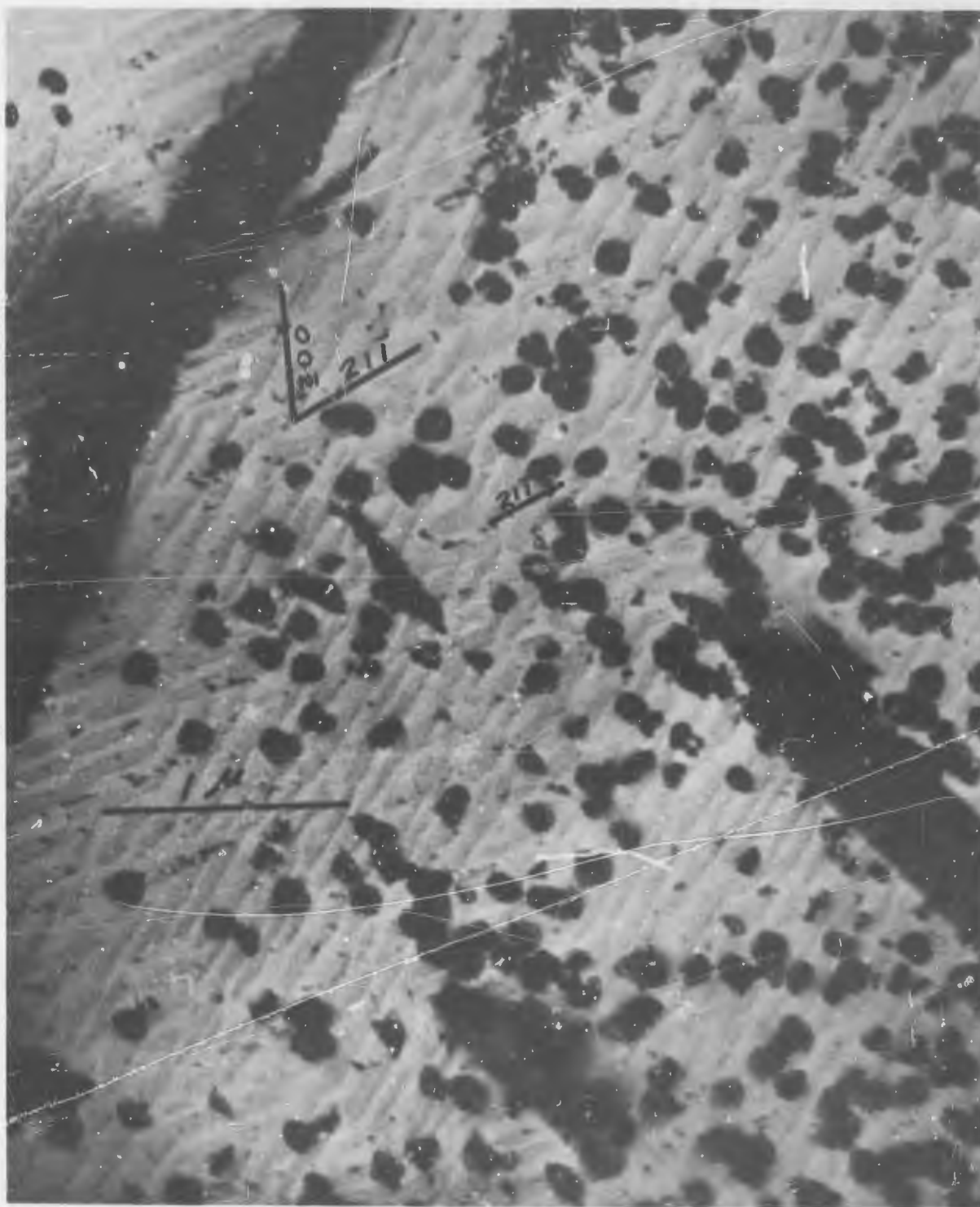
FIGURE 59. Transmission Electron Micrograph of VAM-98 (Cb-22W-2Hf-0.05C-0.04N) Solution annealed 1 hour at 1800°C and helium cooled; plus aged 7 hours at 1100°C. 120 foil showing coherent precipitates.
