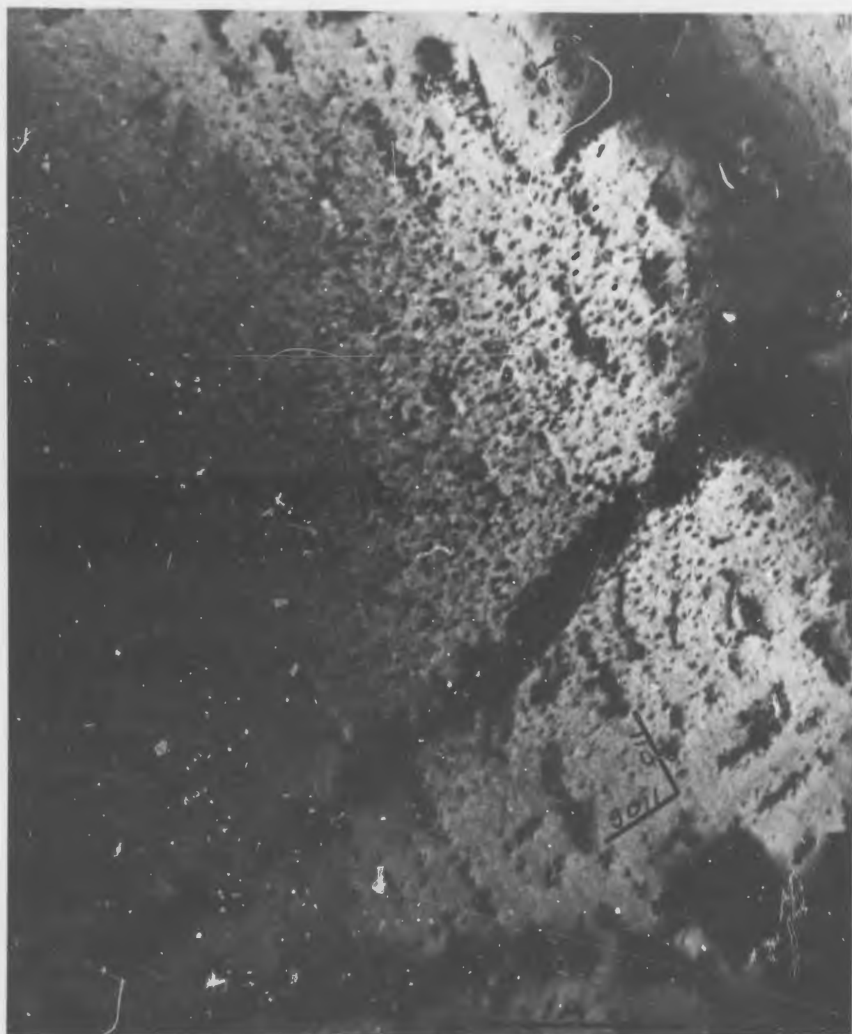
FIGURE 54. Transmission Electron Micrograph of VAM-98 (Cb-22W-2Hf-0.05C-0.04N) Solution annealed 1 hour at 1800°C and helium cooled; (001) foil showing some coherent precipitation.
