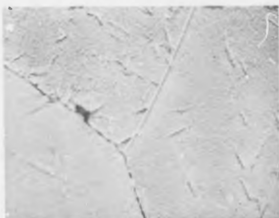
(g) (18,708) Solution Heat Treated+ 1 Hr. at 1200°C
