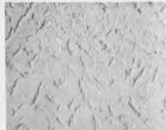
(f) (18,707) Solution Heat Treated+ 1 Hr. at 1300°C
