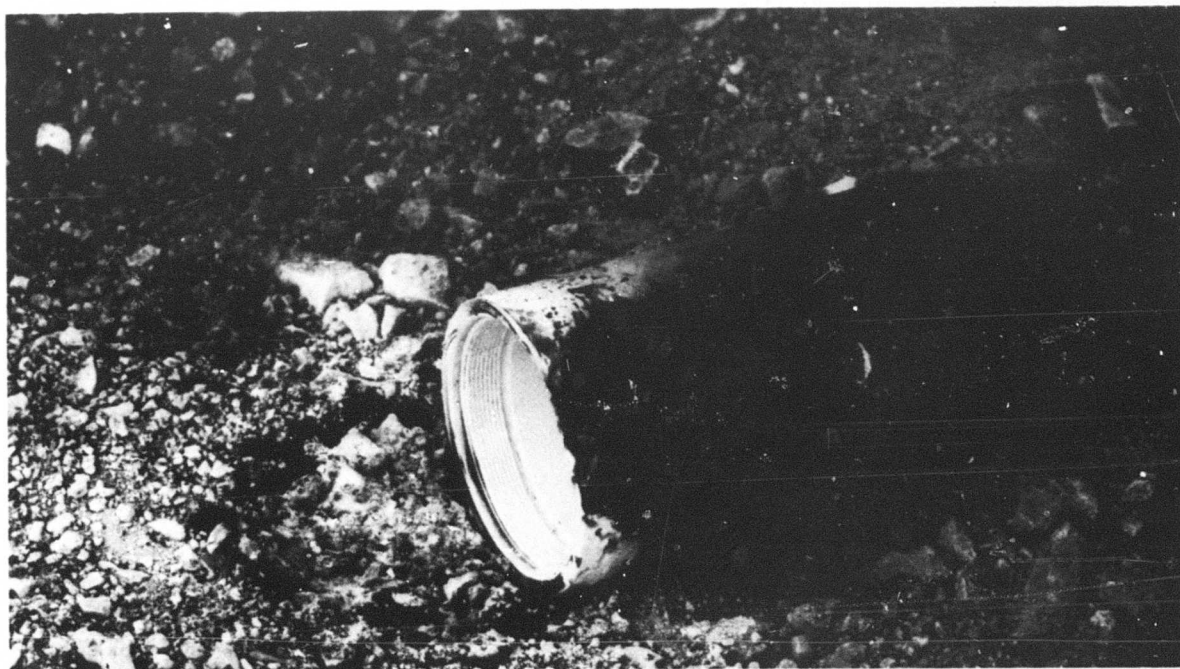
FIG. 7. View of TM-4C Motor Case After 20 mm Bullet Impact. The warhead separated from the motor, but was not damaged. The 20 mm projectile remained in the motor and all propellant was consumed.
