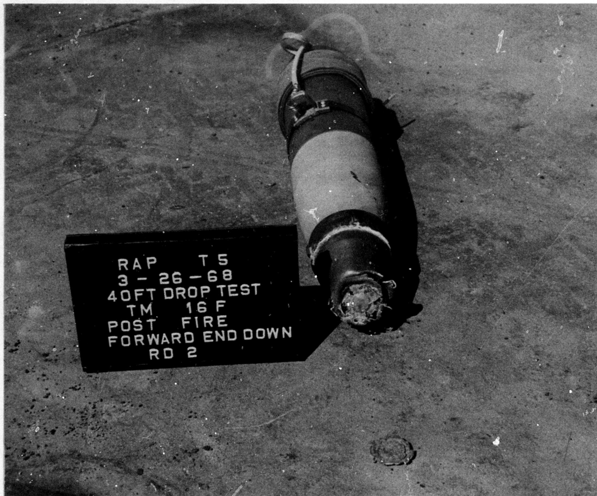
FIG. 3. View of CVT-Fuzed Projectile After Nose-Down 40-Foot Drop (LHL 142878).
