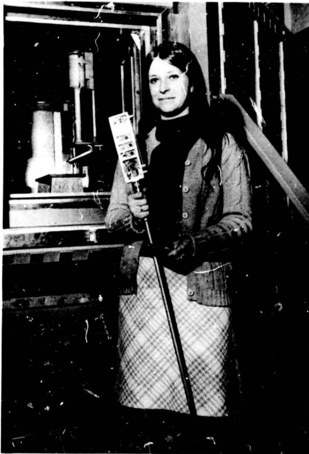
FIGURE 2-12. SQUID ELECTRONIC PACKAGE (COVER REMOVED) AND COAXIAL PROBE. SYMMETRIC SQUID IN GIRL'S LEFT HAND.
