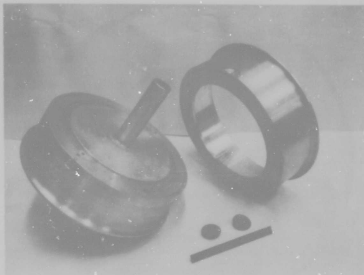
Figure 16. RLA Building-Mandrel, Disassembled
