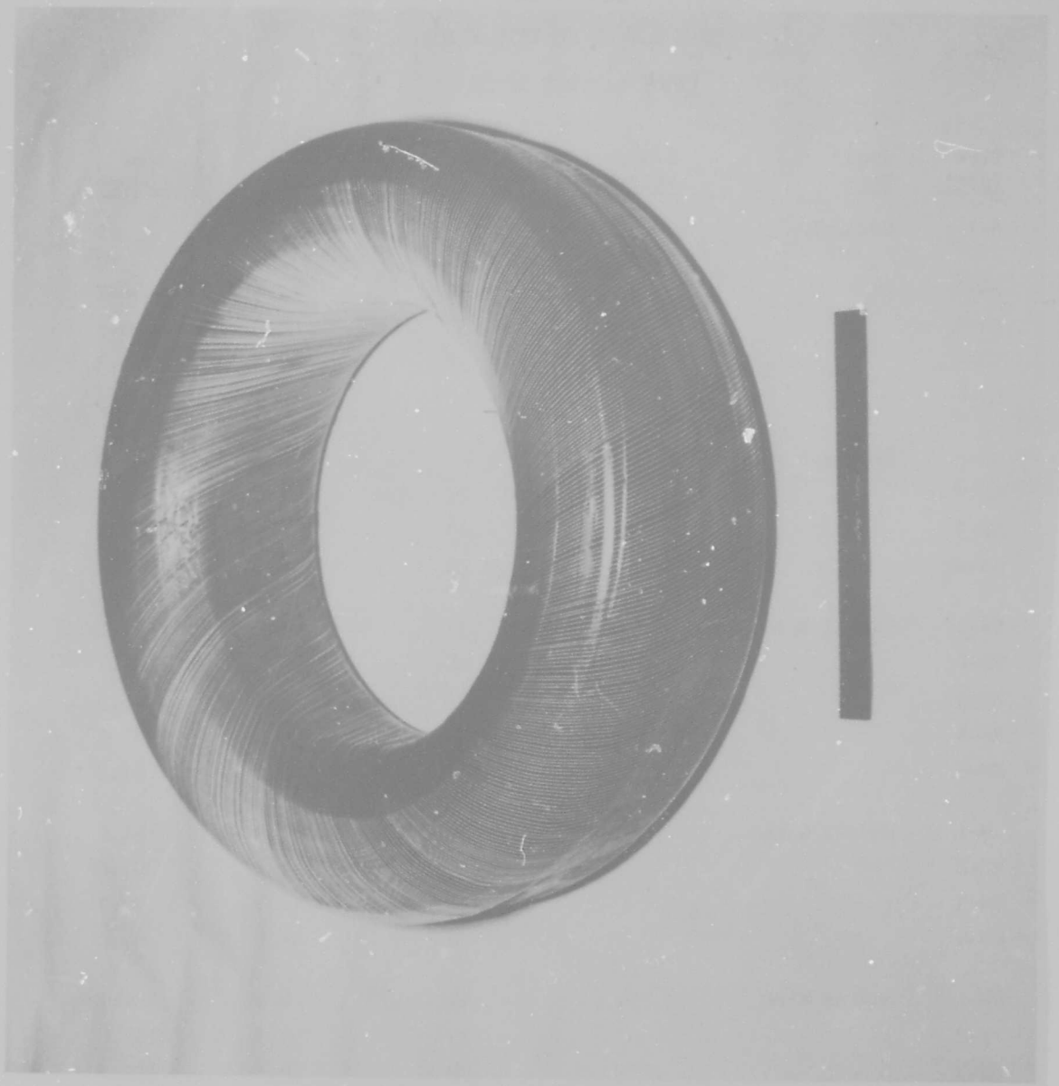
Figure 22. Filament-Wound Geodesic-Nylon Carcass
