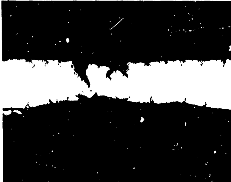
Figure 23. Hastelloy X After a 204-hr Exposure at 1300°F and 20.8 ksi.
