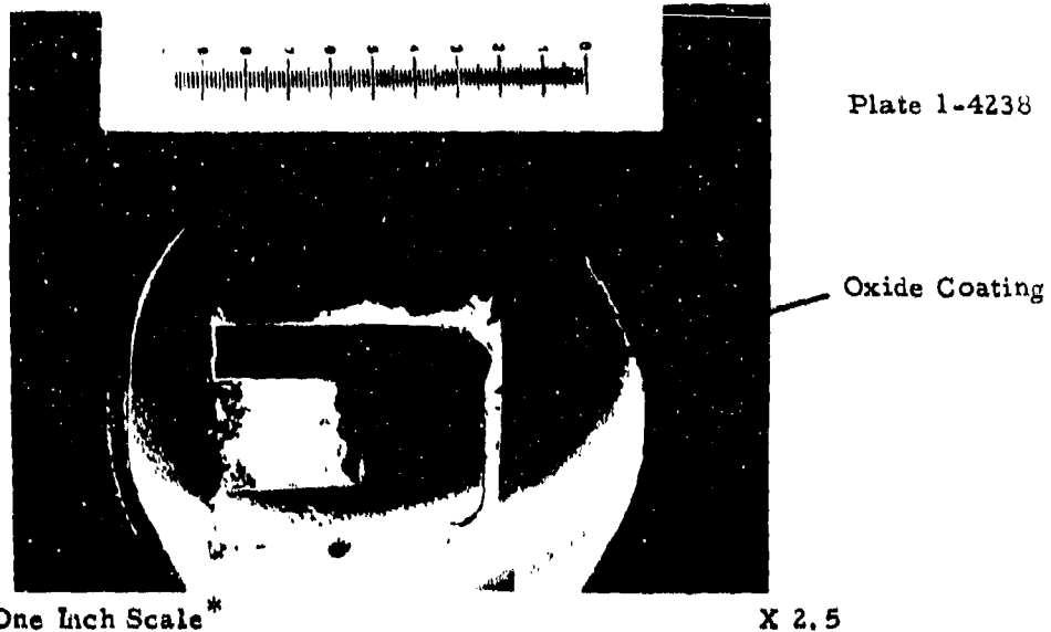
Figure 12. Arc Plasma Test \text{HfB}_{2.1} (A-2)-4M, Surface Temperature 5270^{\circ}\text{F} , Stagnation Enthalpy 5570 \text{ BTU/lb} , Stagnation Pressure 1 \text{ atm} , Cold Wall Heat Flux 760 \text{ BTU/ft}^2 , Exposure Time 1830 \text{ Seconds} , Initial Thickness 557 \text{ Mils} , Final Thickness 286 \text{ Mils} . Hot Face at Right.
